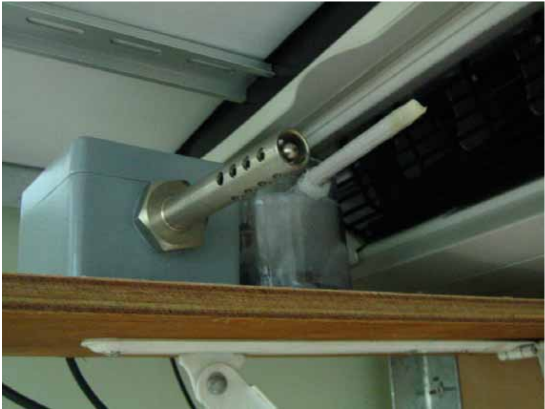
Photo 2 A temperature sensor set for measuring dry- and wet- bulb temperatures
