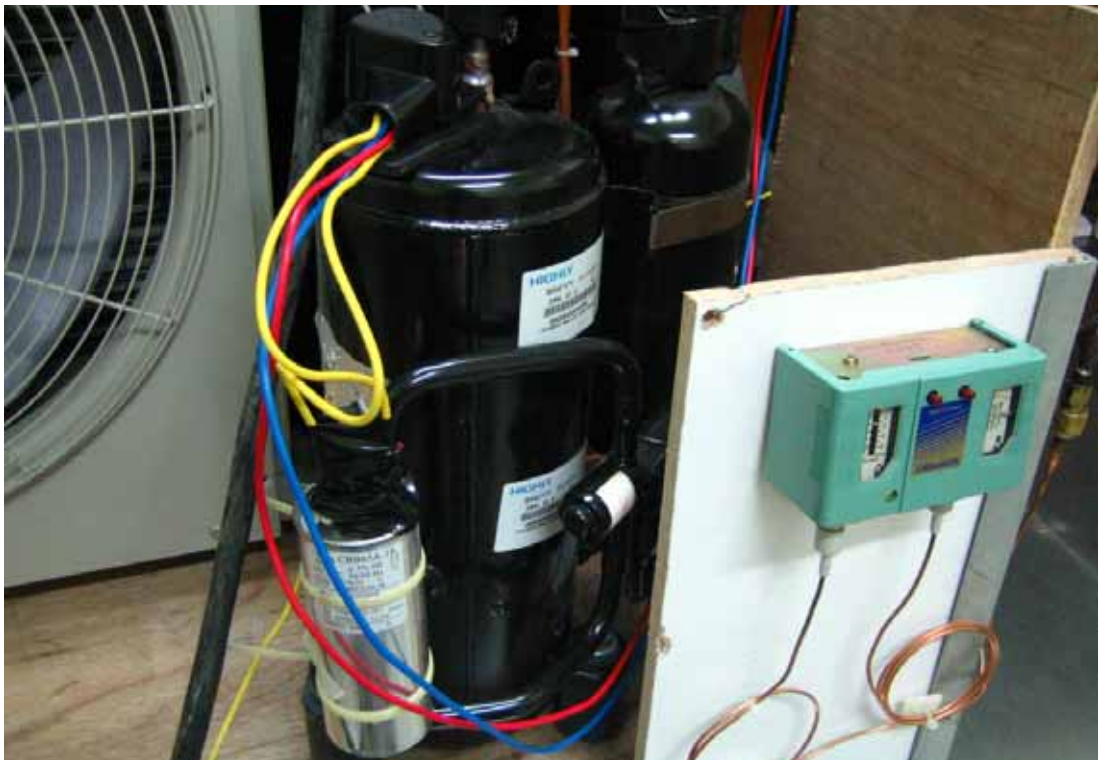
Photo 4 Outdoor unit of the experimental split-type DX A/C system
