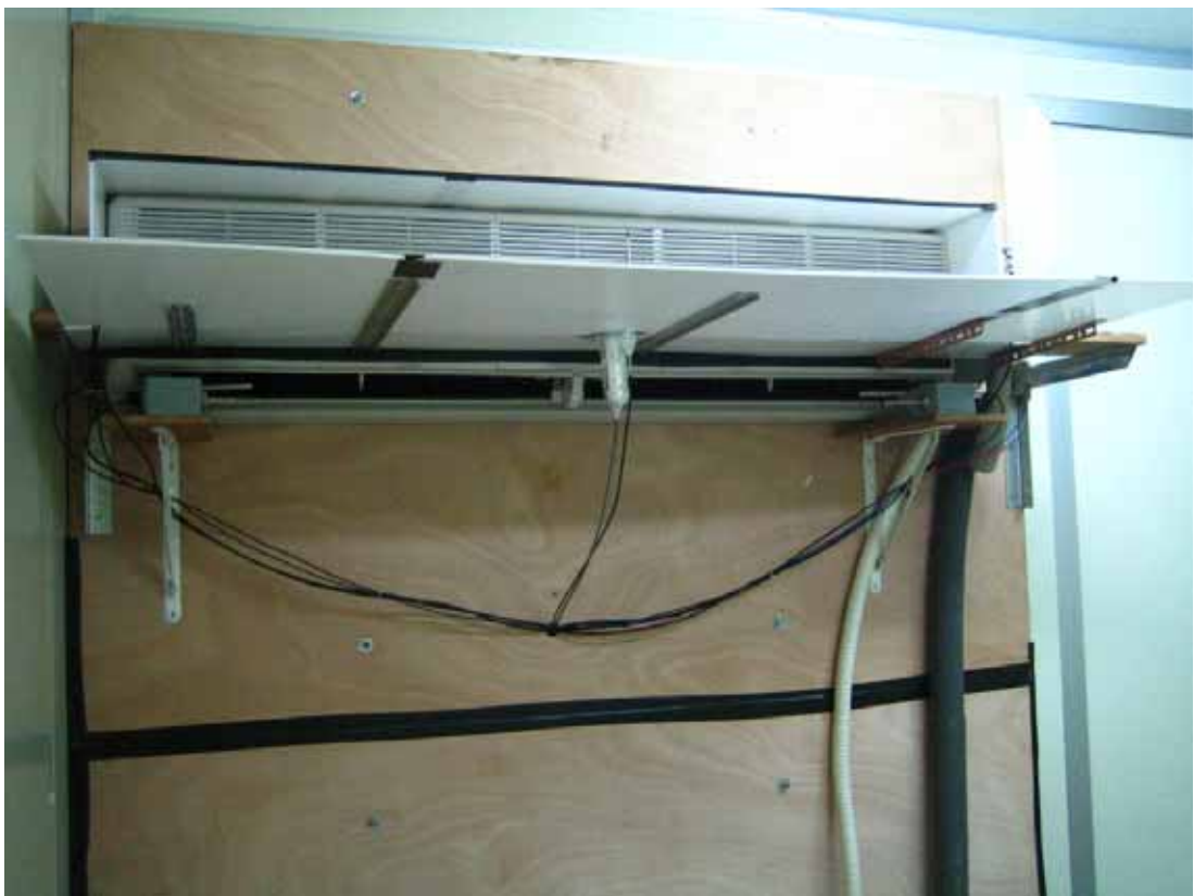
Photo 1 Indoor unit of the experimental split-type DX A/C system
