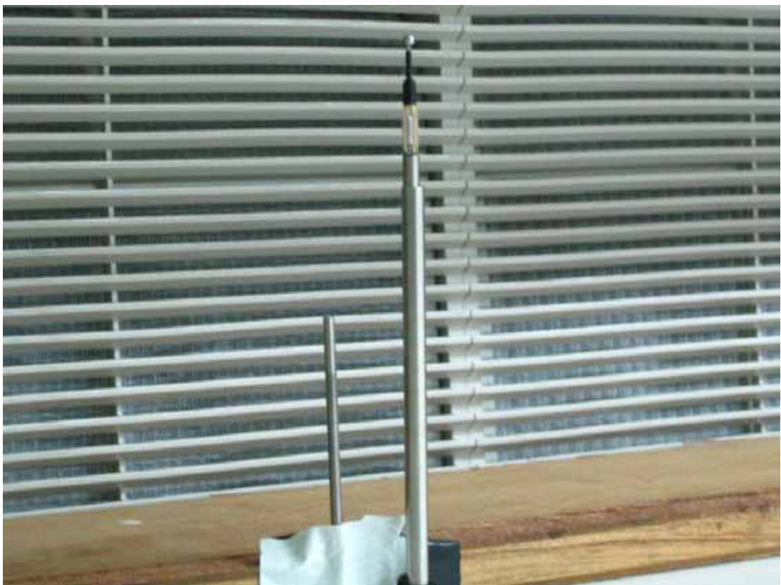
Photo 3 The velocity transducer and temperature sensor
