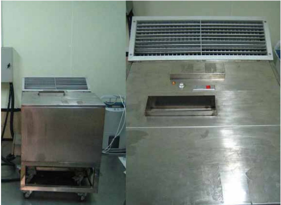
Photo 6 The sensible heat and moisture load generating unit
