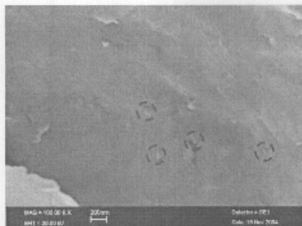
Fig. 2. SEM of the nanoclay composite with 5 min sonicating time at 4 wt.% of nanoclay content.
