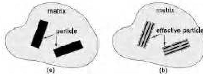
Figure 2.3 Illustration of the “matrix” and “particle” domain in (a) conventional composite and (b) nanocomposite (Captured from Sheng N. et. al., *Polymer*, 45, 487-506; 2004)
