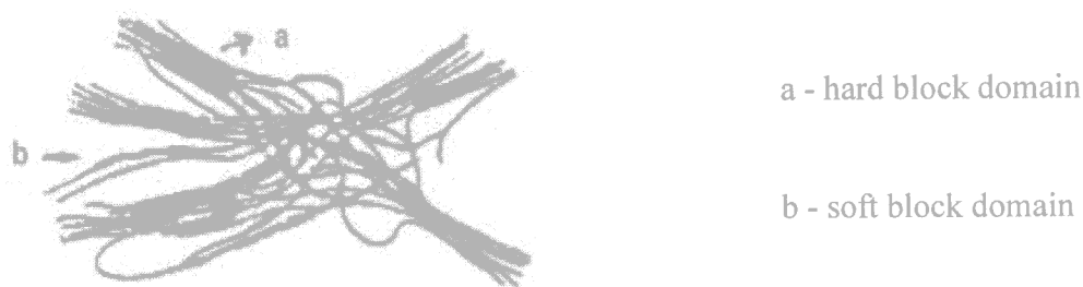
Figure 2.3: Polyurethane with Segmented Domain Structure (Adapted with permission from Vilar Polyurethanes, http://www.poliuretanos.com.br/ [26])
