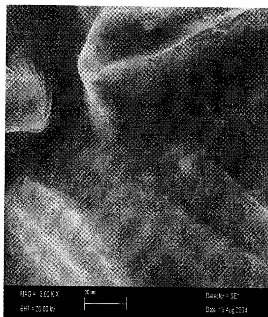
Figure 7.3: SEM image of coated fabric with 0.25 % of MWNT content SPU
