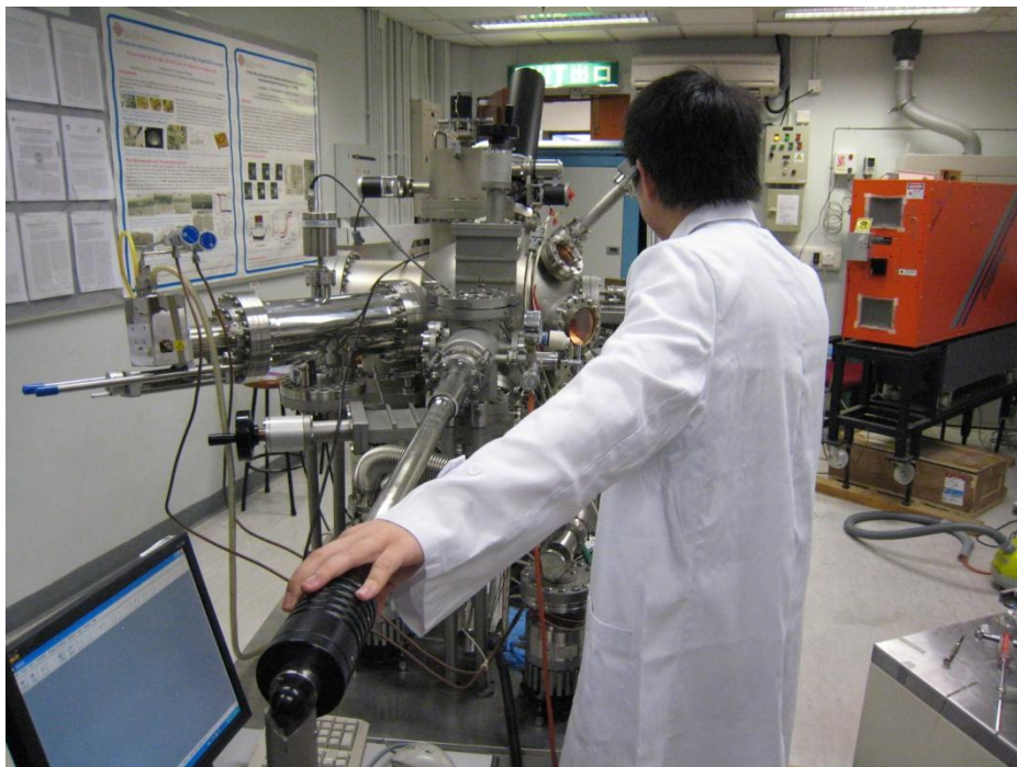
Fig.3.1 Setup of Laser-MBE system used in our experiment.
