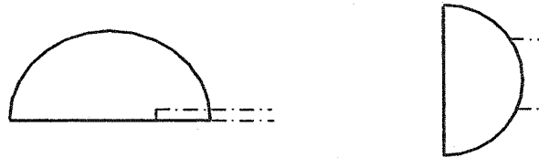
(a) Parting plane at bottom face (b) Parting plane through axis
