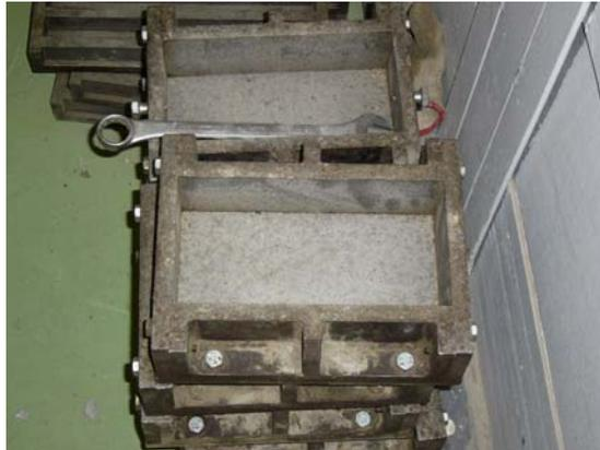
Figure 3.6 Indention mould for paving blocks
