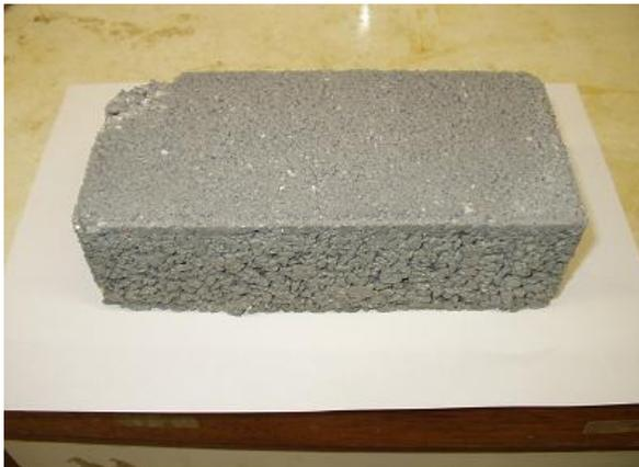
Figure 7.13 Self-designed photocatalytic block
