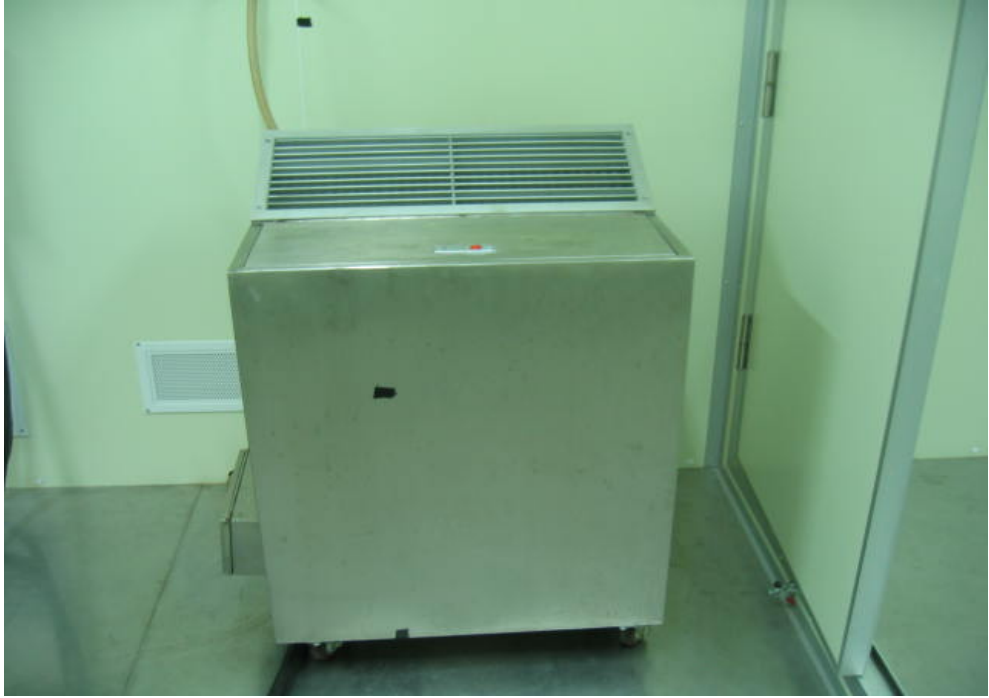
Photo 5 Load generation unit inside conditioned spaces
