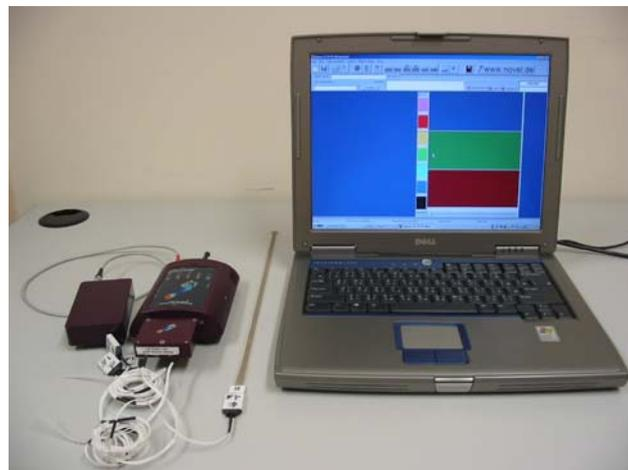
**Figure 5.2a** The Pliance X System for interface pressure monitoring
