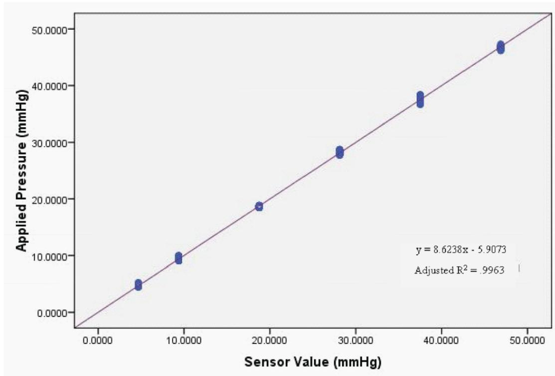
Figure 3.4 Association between sensor output and applied pressure
