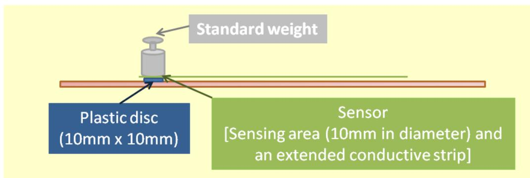
Figure 3.3 Sketched experimental setup for linearity, repeatability and drift tests
