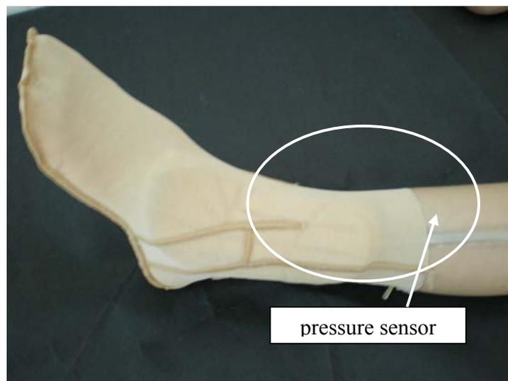
**Figure 5.2b** Measurement of the interface pressure with the Pliance X System Sensor inserted underneath the pressure garment and padding
