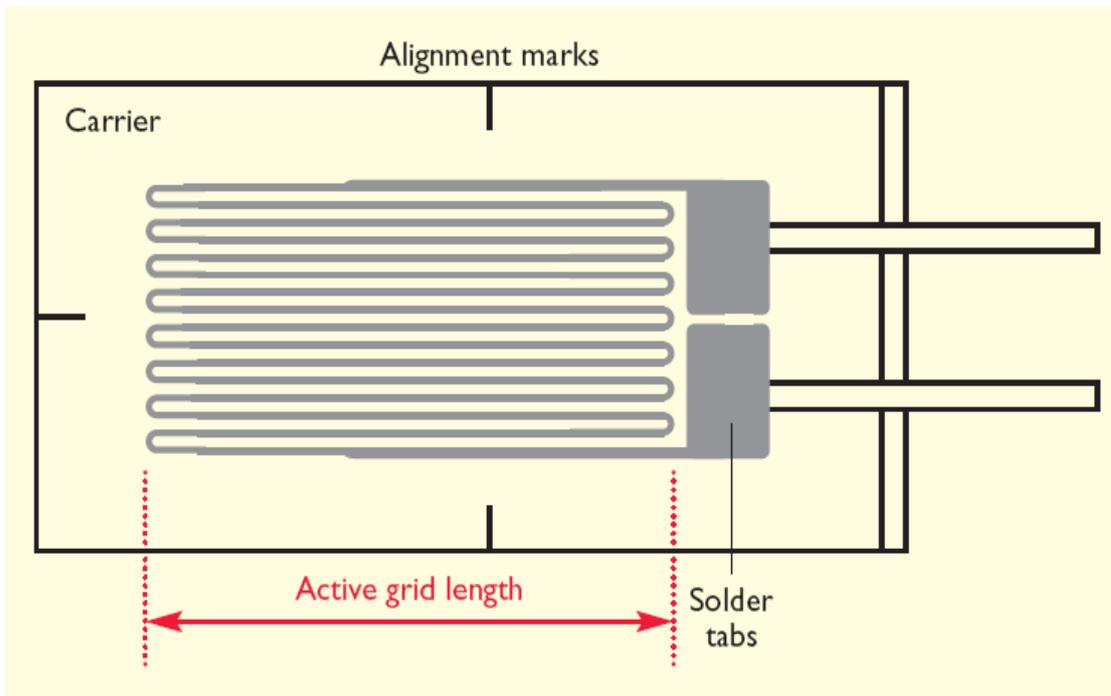
Figure 3.1 Metal wire bonded strain gage (Bethaves, 2002)
