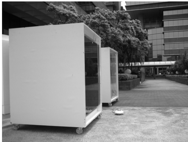
Figure 3.11 Outdoor test facility for DSPV façade and the conventional façade with internal curtain
