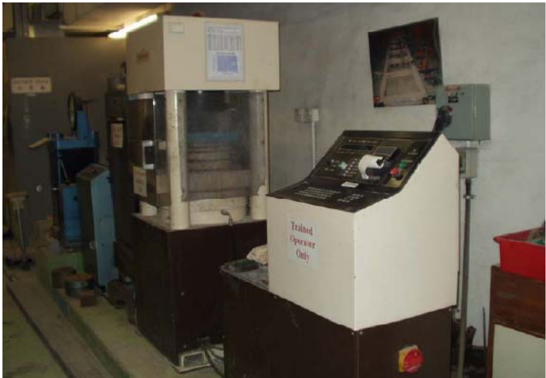
Figure 3.11 Denison compression machine
