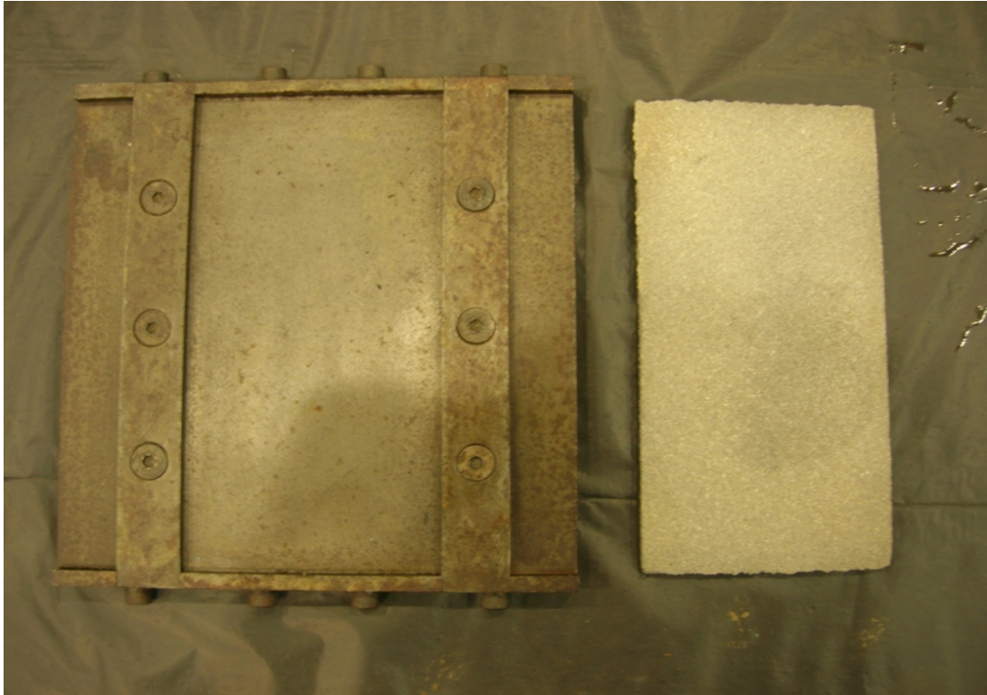
Figure 3.1 Steel mould and surface layer sample
