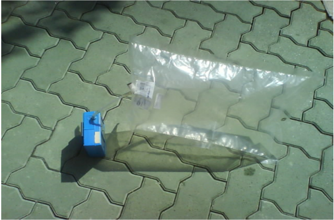
Figure 3.14 Air sampling at ground level
