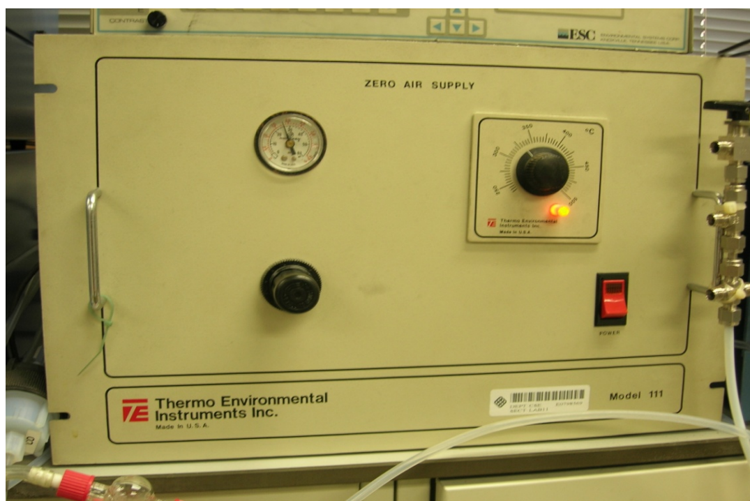
Figure 3.3 Zero air generator
