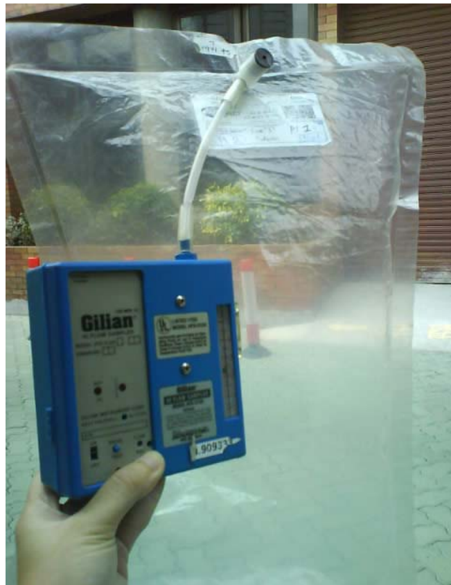
Figure 3.15 Air sampling at breathing zone
