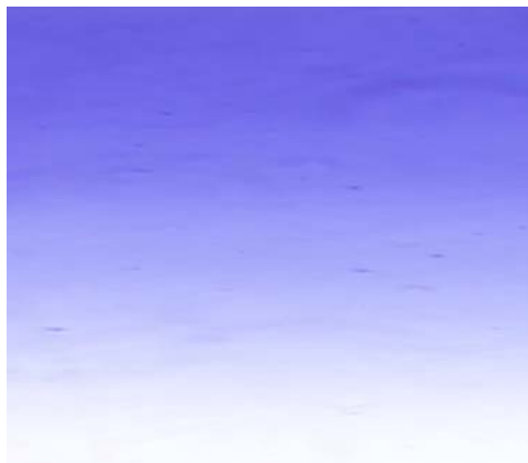
Figure 5.10 Gradient in the microfluidic network of flow rate 0.5 ml/hr
