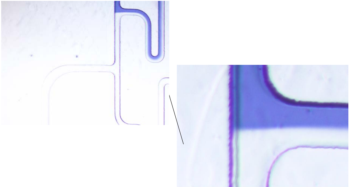
Figure 5.9 Mixing channel in the microfluidic network of flow rate 0.5 ml/hr
