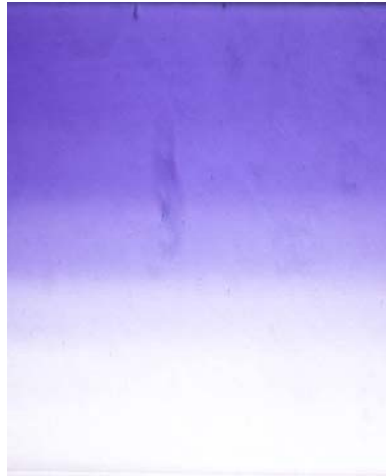
Figure 5.14 Gradient in the microfluidic network of flow rate 2 ml/hr
