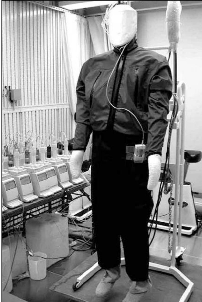
**Figure 2-11. Sweating thermal manikin KEM (Fukazawa et al., 2004)**
