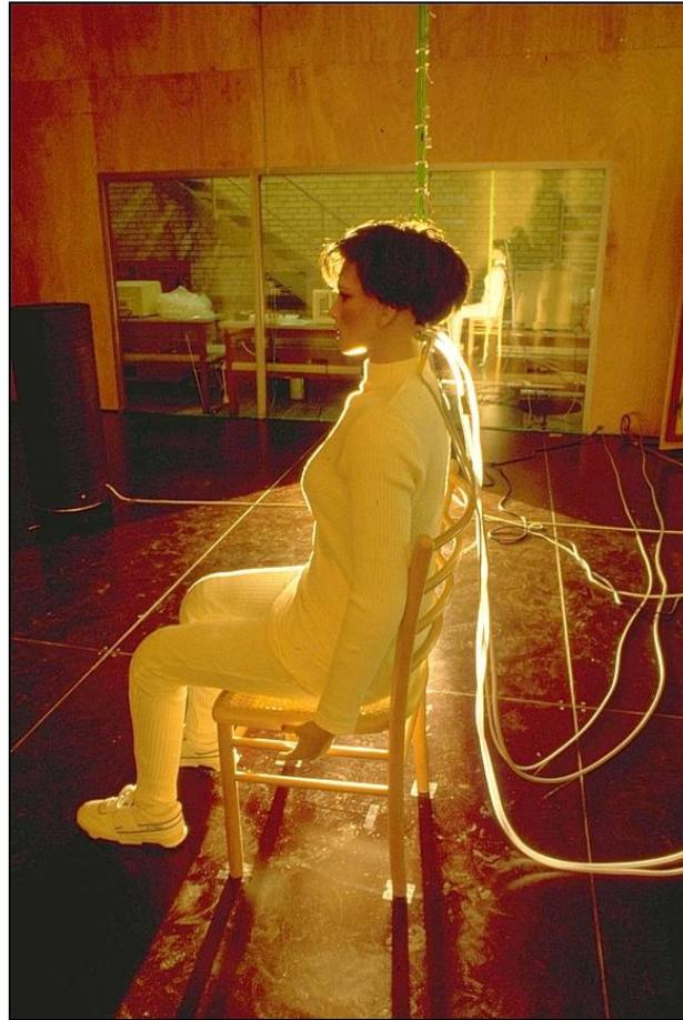
**Figure 2-13. Non sweating seating breathing thermal manikin developed at Danish Technical University**
