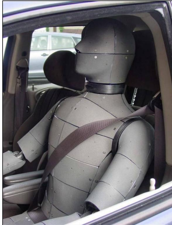
**Figure 2-15. The seated sweating and breathing thermal manikin Adam (Rehn, 2004)**
