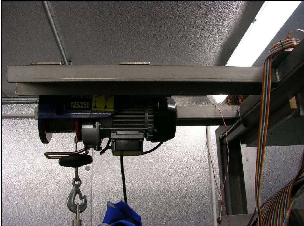
**Figure 3-1. The movable lifting up machine for changing manikin postures, skins and clothing**
