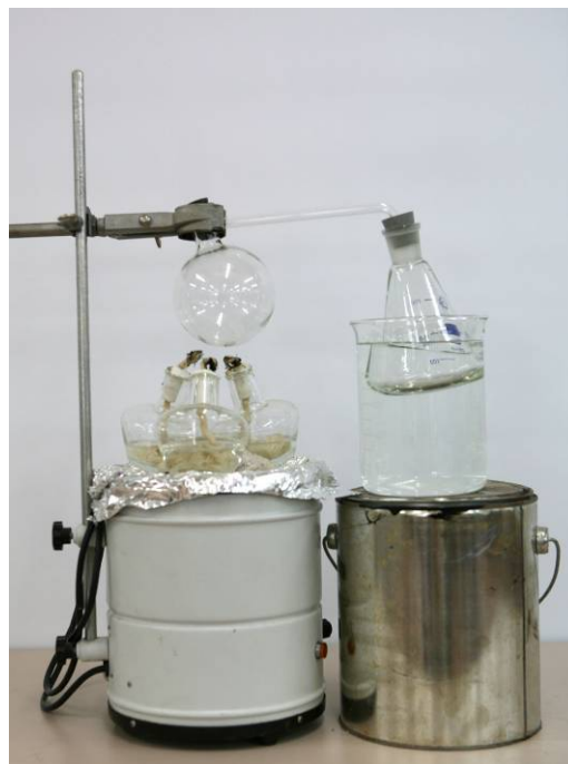
Figure 2.8 Distillation Flask and Associated Apparatus
