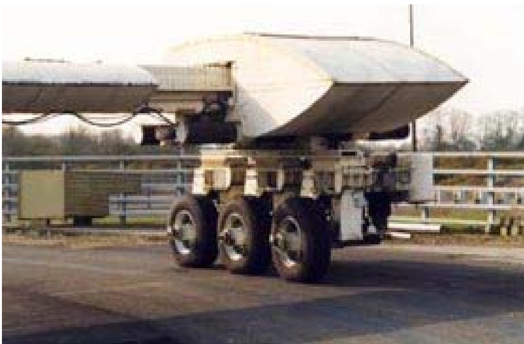
Figure 6.4 Triple-tyre Loading System (Source from Website)
