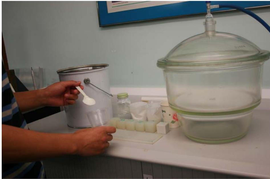
**Fig. 5.1.** Photos of production of ASR: (a) mixing silicon gel, firm agents and oil; (b)
