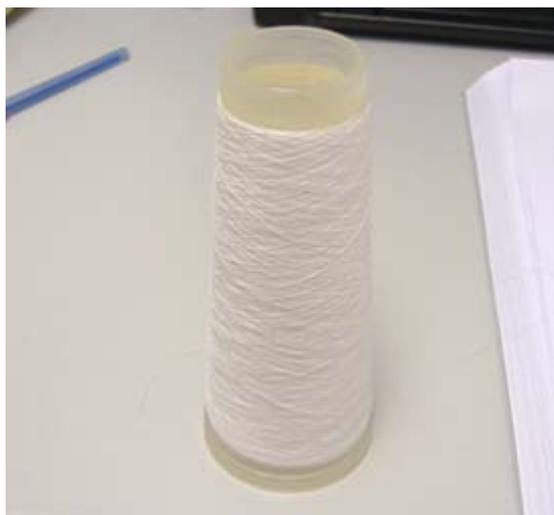
Figure 9.2 PBA -based SMFs prepared by wet spinning
