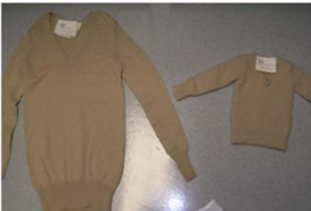
Figure 1.10 Improved dimensional stability of SMP treated wool garments [109]
