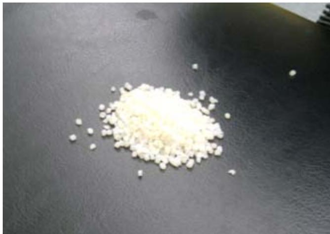
Figure 4.2 PCL-based SMPU chips
