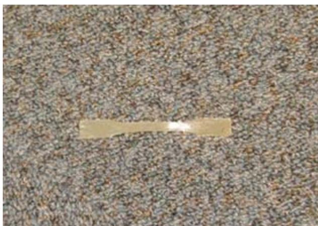
Figure 9.11 Dumb-bell shape specimens of SMPU film
