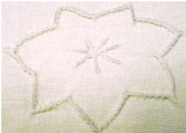
Figure 1.8 The pattern after 2 times washing [107]
