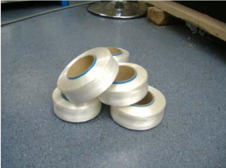
Figure 4.7 PCL-based SMFs prepared by melt spinning
