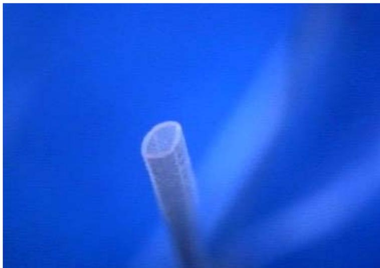
Figure 6.1 Cross-section image of the prepared hollow fiber
