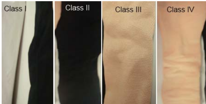
Figure 6-17 Stocking samples after 25 cycles of flexing on Instron
