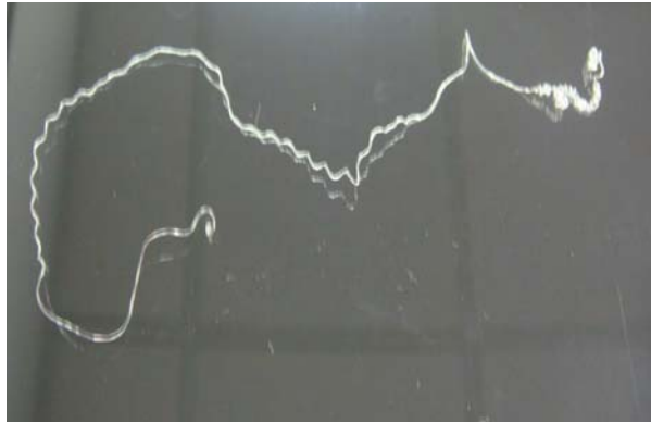
Figure 5-15 Shape memory filaments reformed to a ringlet structure after pre-setting
