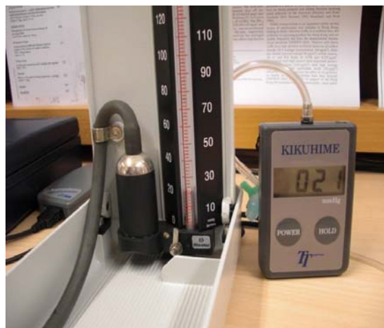
Figure 3-4 Calibration of Kikuhime sensor using sphygmomanometer
