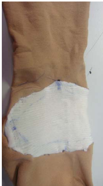
Figure 6-18 Shape memory stockings sample after 25 cycles of flexing on Instron
