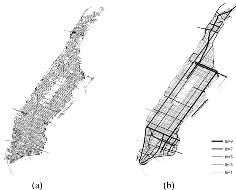
**Figure 7.8** Road network in New York County and its skeletons at 5 scales
