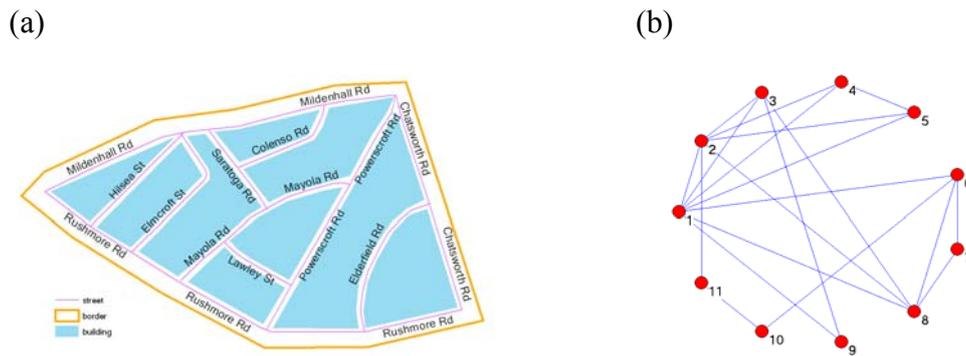
**Figure 1.1** A sampled road network and one of its graph representations
