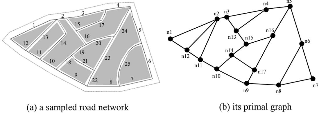
**Figure 2.7** A sampled road network and its primal graph
