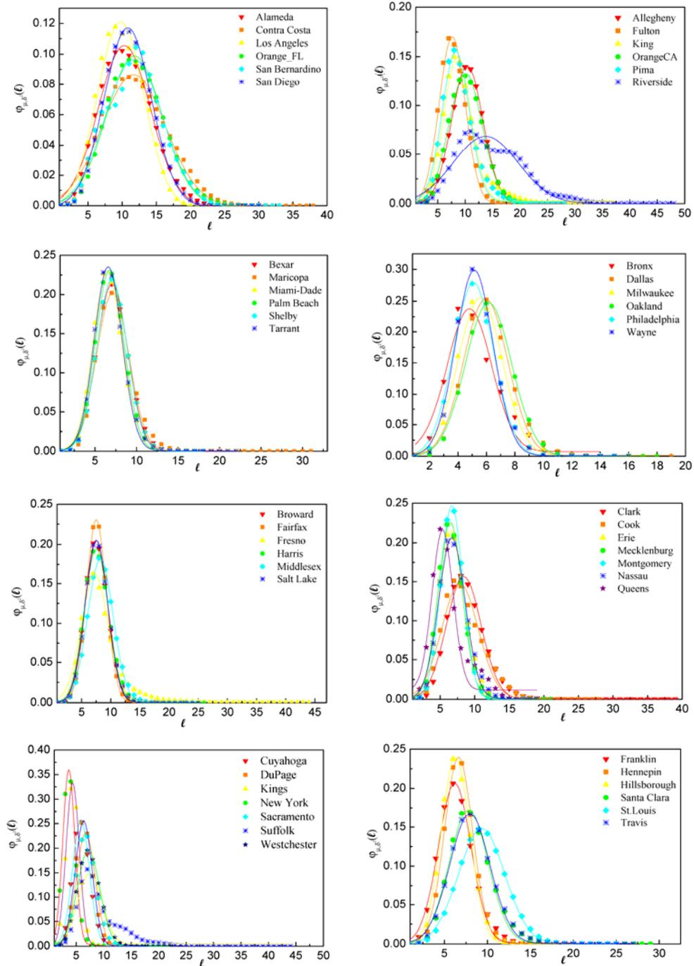
**Figure 3.7** Distributions of the lengths of the shortest paths in 50 road networks
