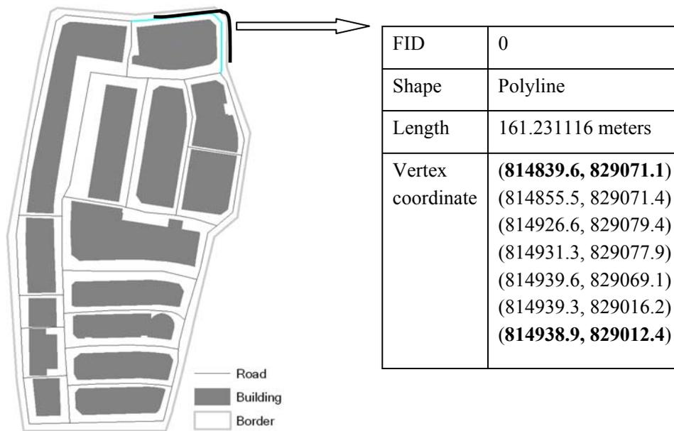
**Figure 2.6** A road in a housing estate and its geometric representation
