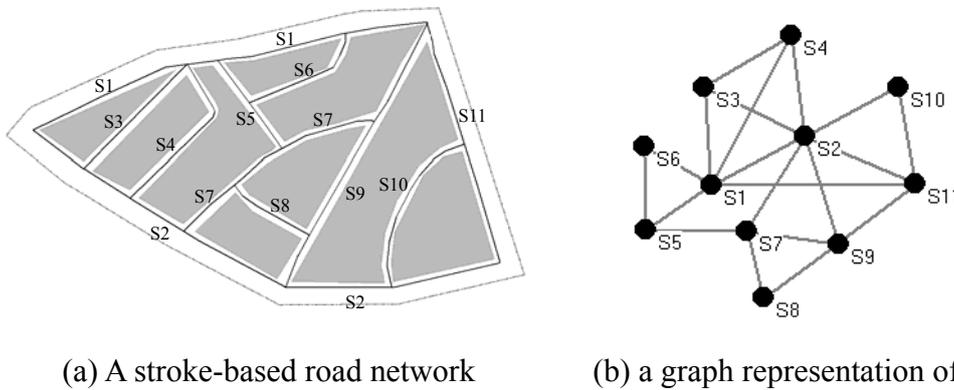
**Figure 3.2** A stroke-based road network and its graph representation
