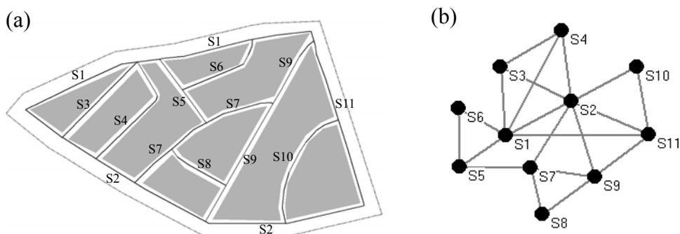
**Figure 4.2** A sampled road network and its graph representation
