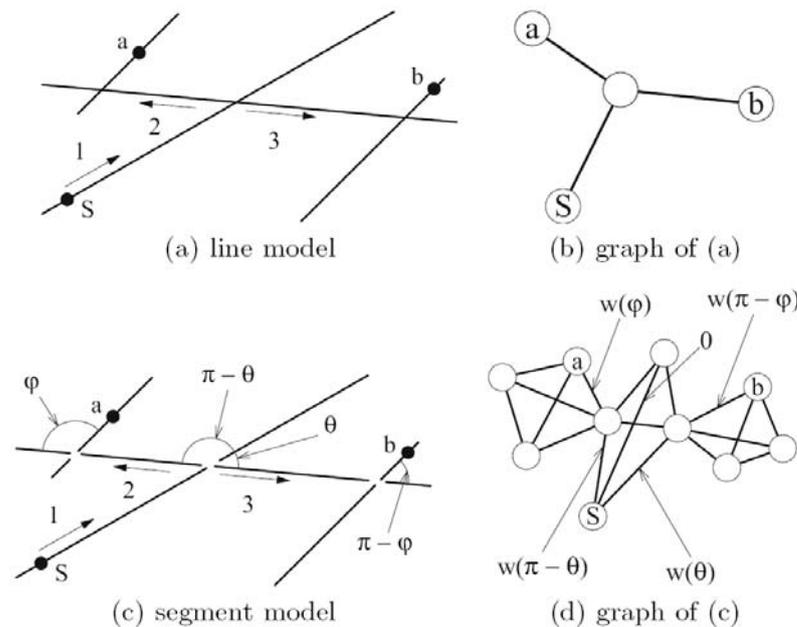
**Figure 2.10** A sampled road network and its disaggregated model (Hillier and Iida 2005)
