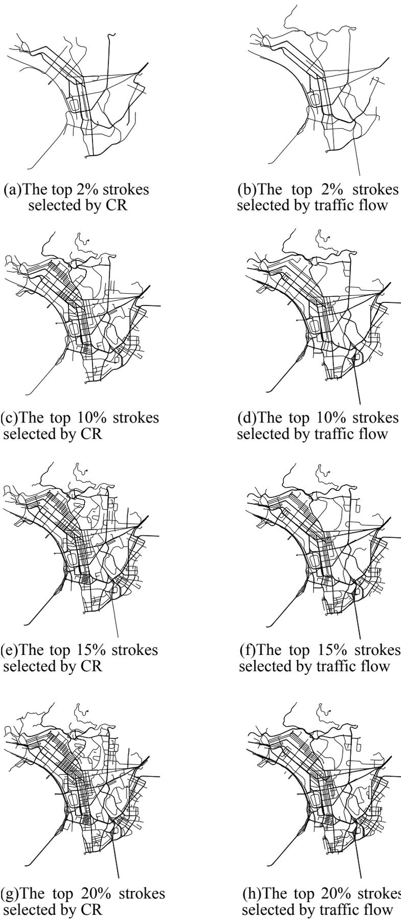
**Figure 5.7** Strokes selected by CR or traffic flow of the KSY road network
