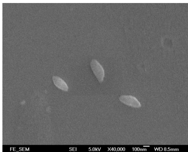
Figure 3.14 FE-SEM image of the ellipsoidal particle with an aspect ratio ( \Lambda ) of around 3 (major axis a = 400 nm, minor axis b = 130 nm)
