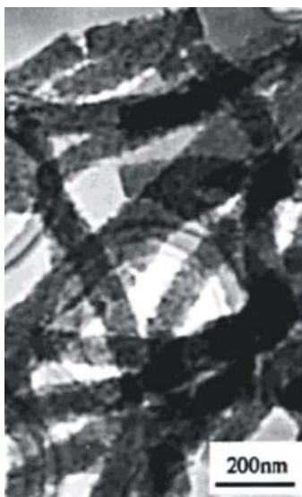
Figure 1.20 TEM image of self-assembled polyaniline nanotubes. 94
