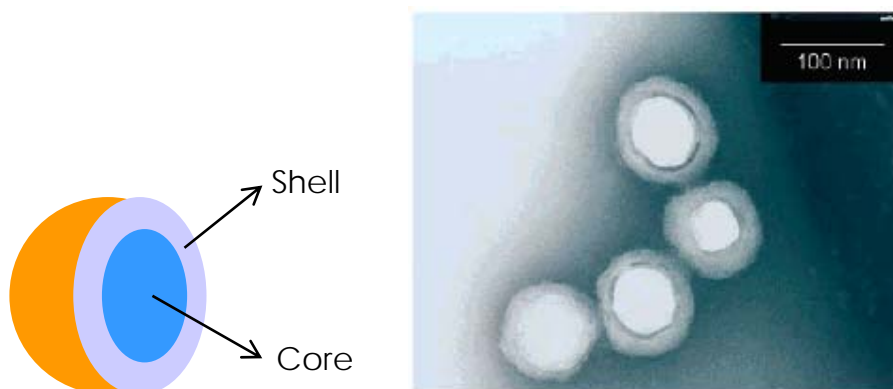
Figure 1.32 Illustration of typical core-shell nanoparticles and TEM image of PEI/PMMA core-shell nanoparticles. 195
