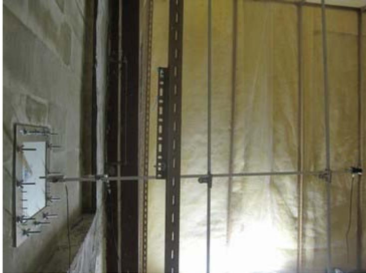
**Figure A.7 Microphones setup in the receiving chamber for measuring the radiated (transmitted) sound field**
