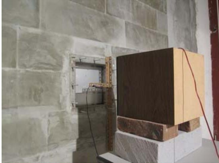
**Figure A.5 A loudspeaker box as a plane wave source**
