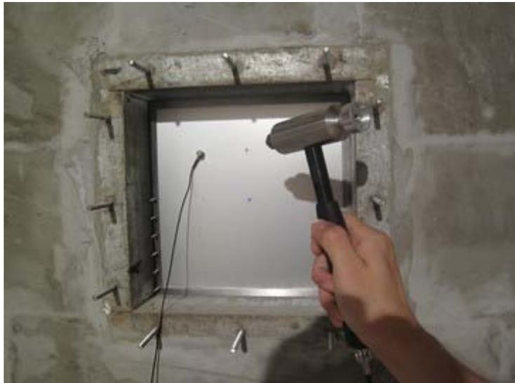
**Figure A.6 A hammer as an impact source**
