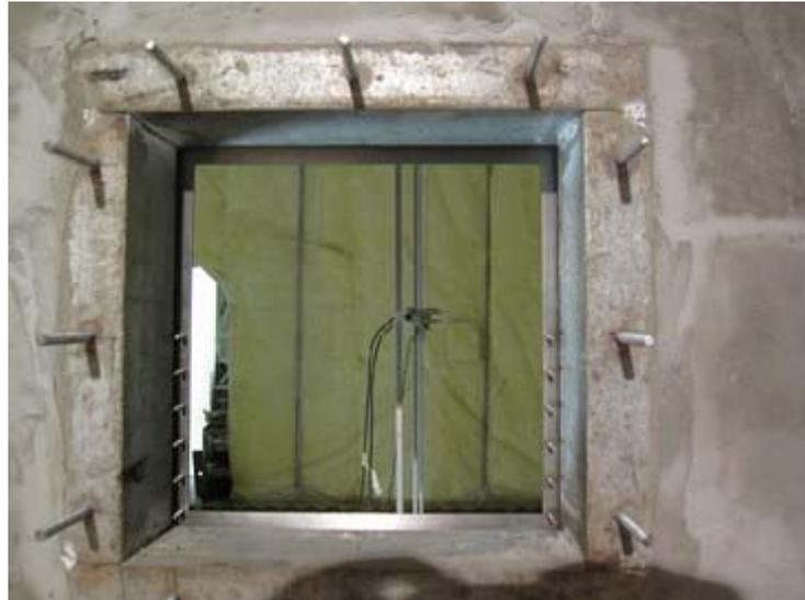
**Figure A.2 The hole of the common wall between the two chambers**
