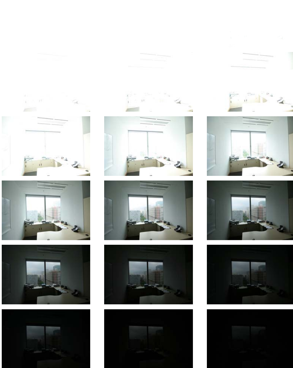
Figure 6.13 Eighteen LDR photographs of multiple exposures of a test cellular office as the first scene (first row left to right: 30 s, 15 s, 8 s; second row left to right: 4 s, 2 s, 1 s; third row left to right: 1/2 s, 1/4 s, 1/8 s; fourth row left to right: 1/15 s, 1/30 s, 1/60 s; fifth row left to right: 1/120 s, 1/250 s, 1/500 s; sixth row left to right: 1/1000 s, 1/2000 s, 1/4000 s)
