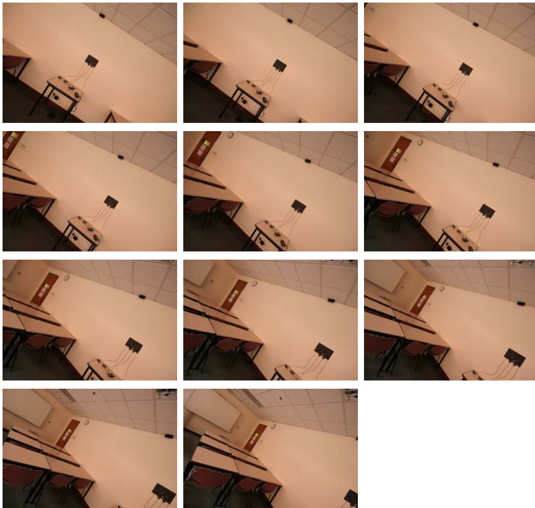
Figure 6.4 The centre of the grey card lies on the diagonal line of the scene when rotating horizontally the 33.7° inclined camera at every 5° from 0 to 50°
