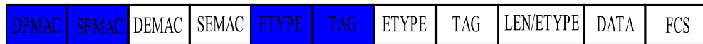
Figure 1.6: Frame formats in Ethernet, MPLS metro network and pure Ethernet metro network
