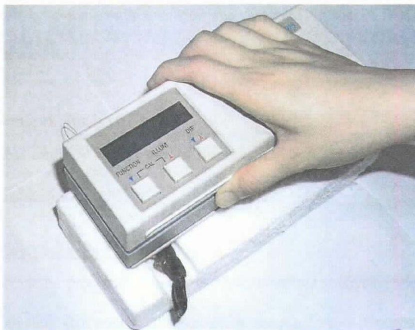
Plate 3.2.3 Measurement of shrimp surface lightness by use of portable Tri-stimulus Reflection Colorimeter.
