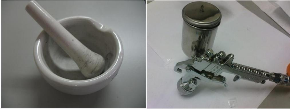
Figure 4.23. Equipments for sample preparation. Left: a mortar and pestle; right: a spray gun.
