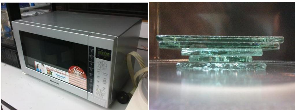
Figure 4.22. Equipments for microwave bonding. Left: a domestic microwave oven; right: a stack of glasses.
