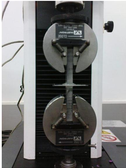
Figure 6.15. Setup of the pulling system for the tensile test.
