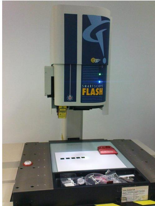
Figure 5.11. Setup of the thickness measurement of CNTs on the spray-coated PC plates.
