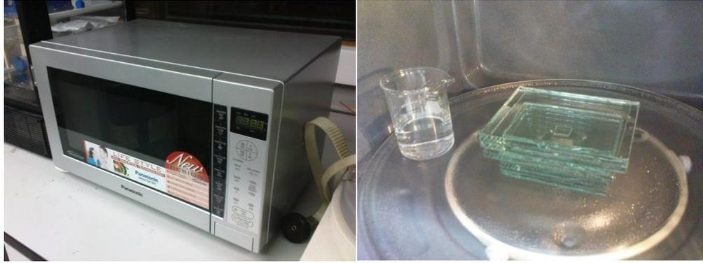
Figure 6.5. Bonding equipments. Left: microwave oven; right: bonding setup inside microwave oven with water loading.
