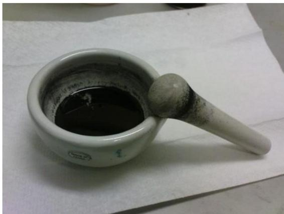
Figure 5.8. Mortar and pestle for grinding CNTs.
