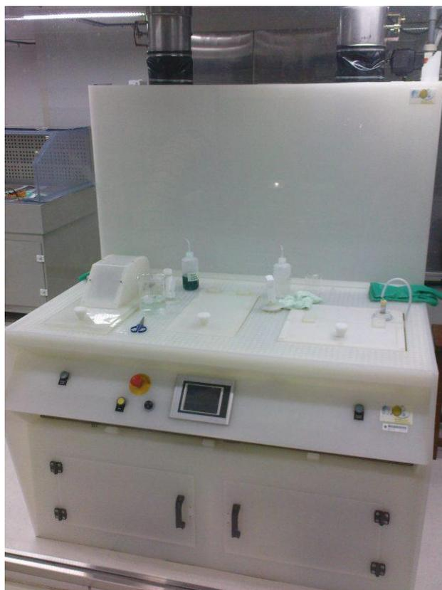
Figure 4.8. Electroforming machine.
