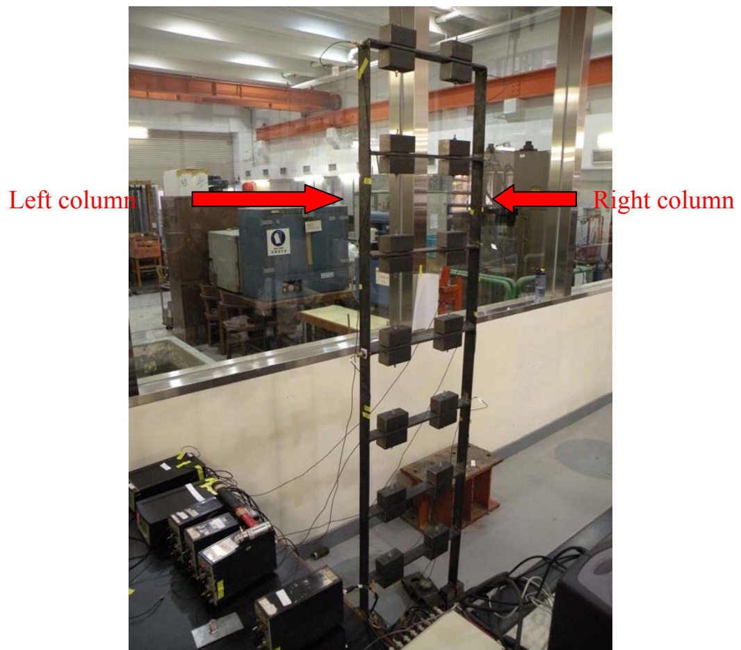
Figure 6.2: The laboratory steel frame model
