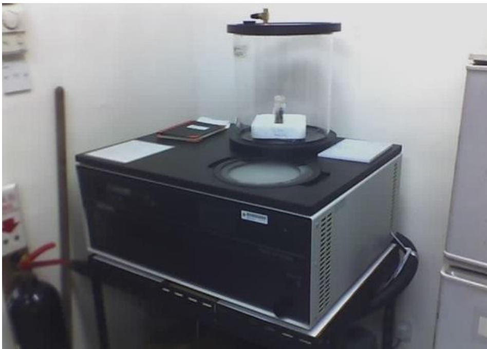
Figure 3.7 The free dryer system
