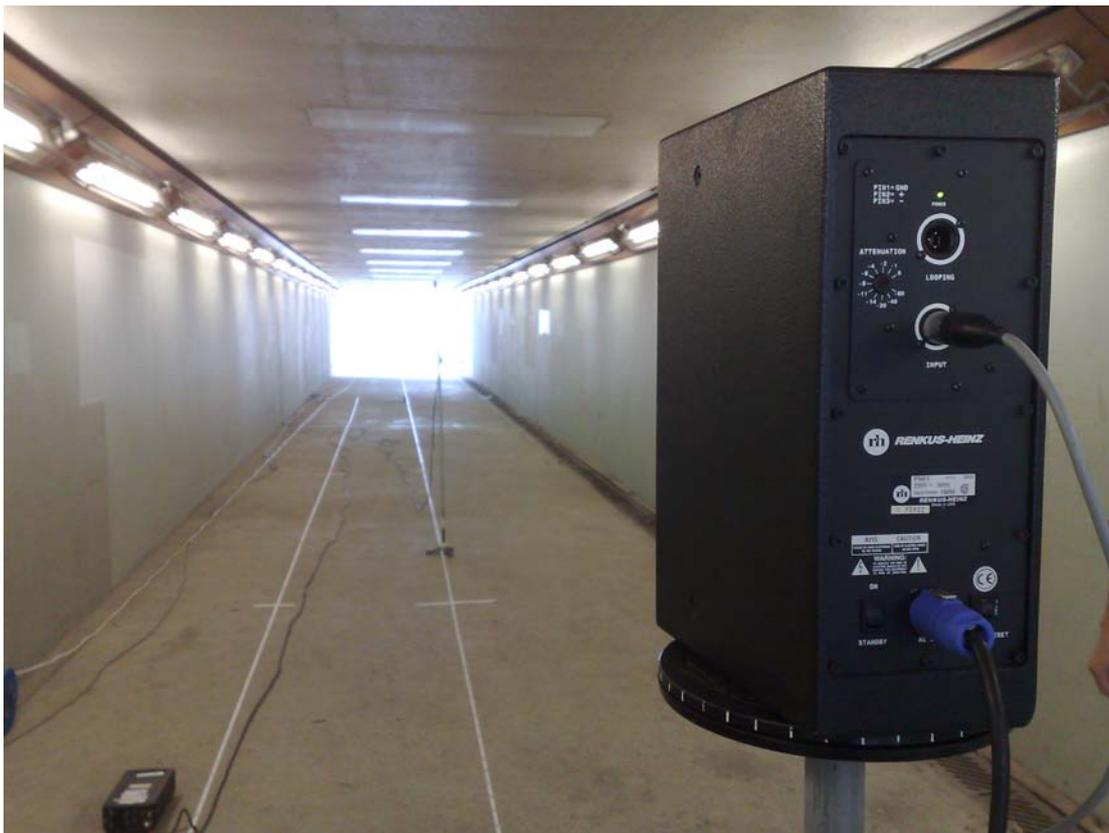
Fig. 3.11: Photograph displaying the experiment setup of the outdoor field measurements. The foreground is the sound source, PN 81 self-powered loudspeaker. The receiver is located in the centre of the photograph.
