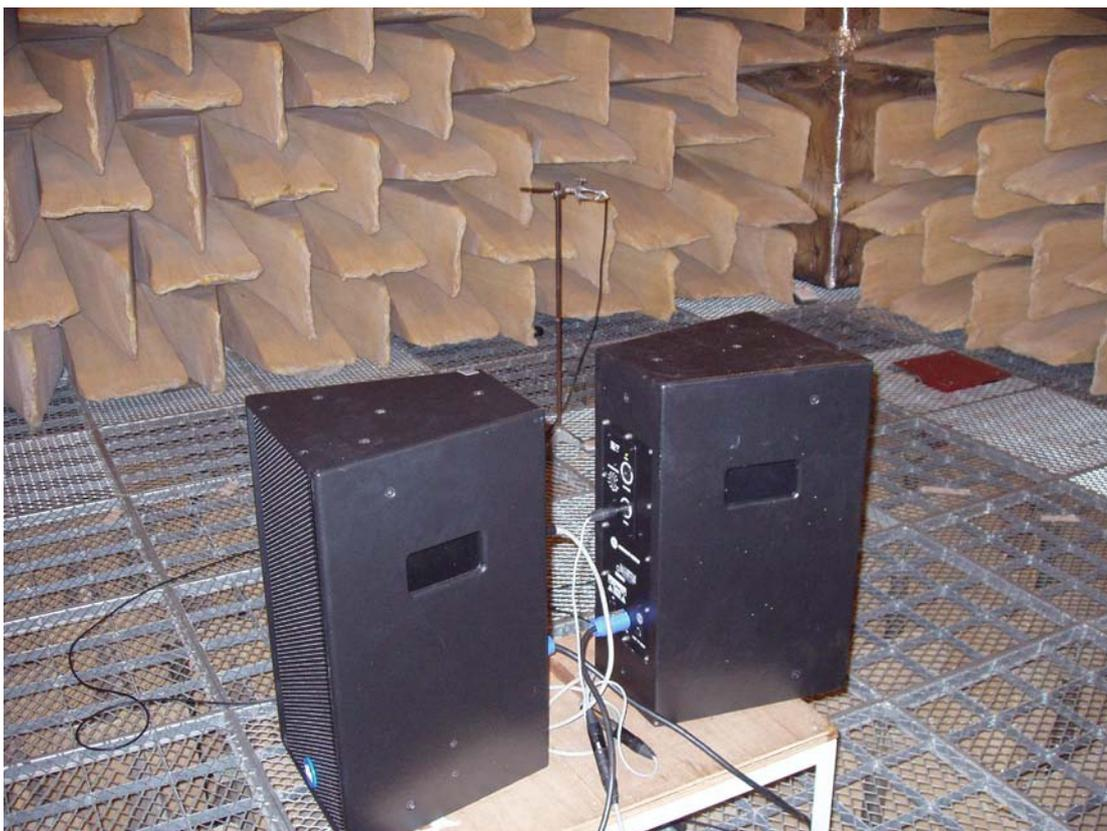
Fig. 6.6: The arrangement of the dipole source constructed by two “Renkus-Heinz” PN 81 self-powered loudspeakers.
