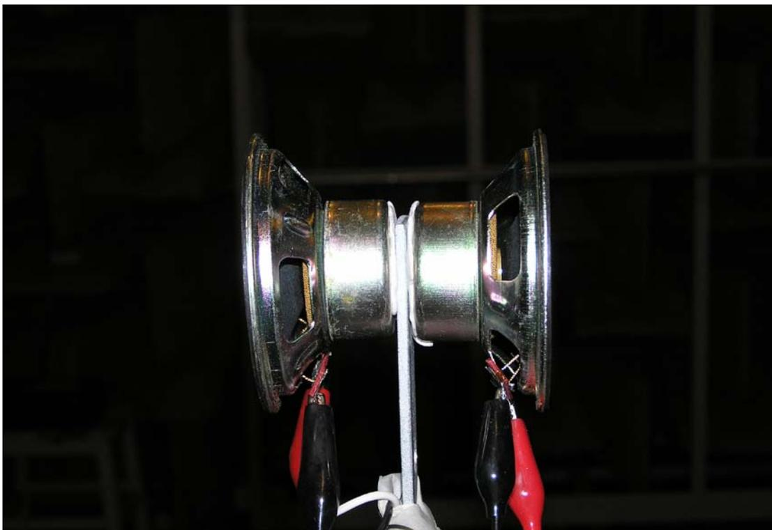
Fig. 6.11: The arrangement of the dipole source constructed by two 5.5" inch un baffled loudspeakers.
