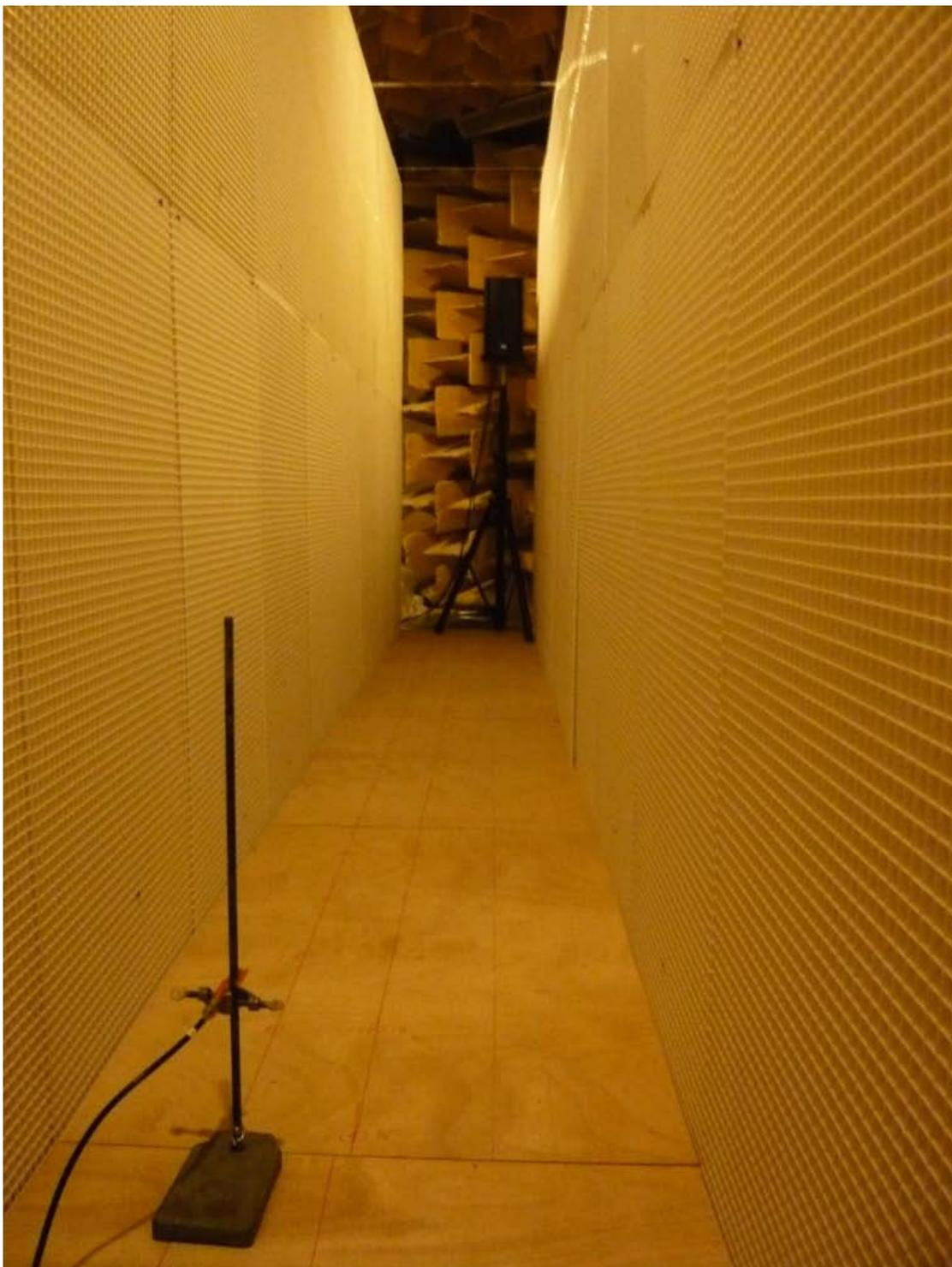
Fig. 2.7: Photograph showing the set-up of the indoor experiment conducted in an anechoic chamber.
