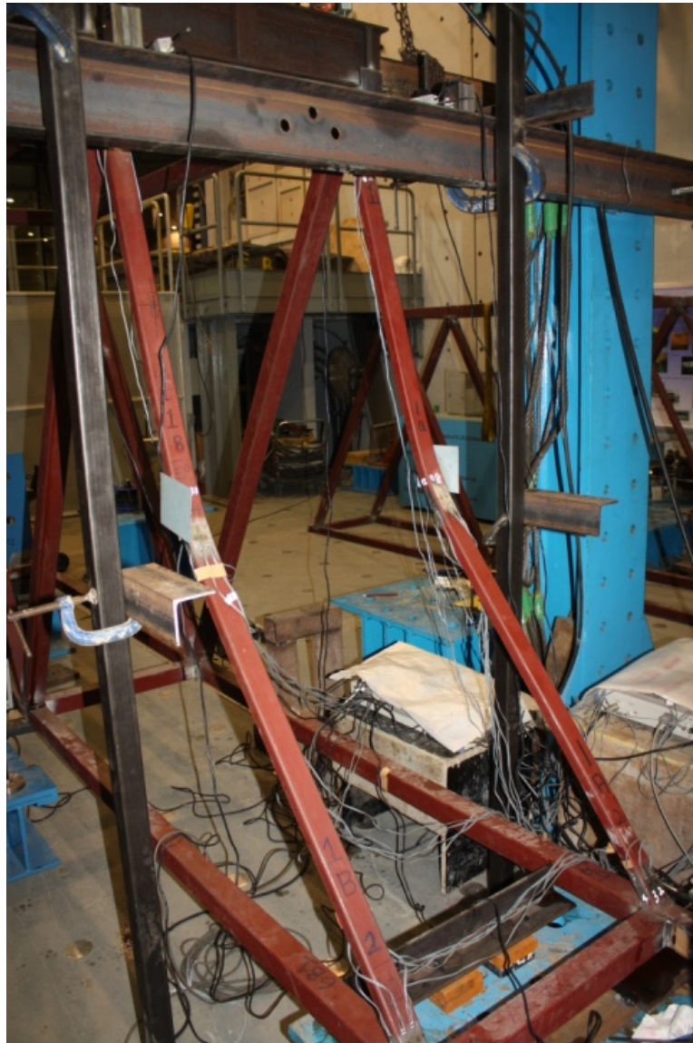
Figure 5.19 Buckling Mode of Set-2 Steel Truss
