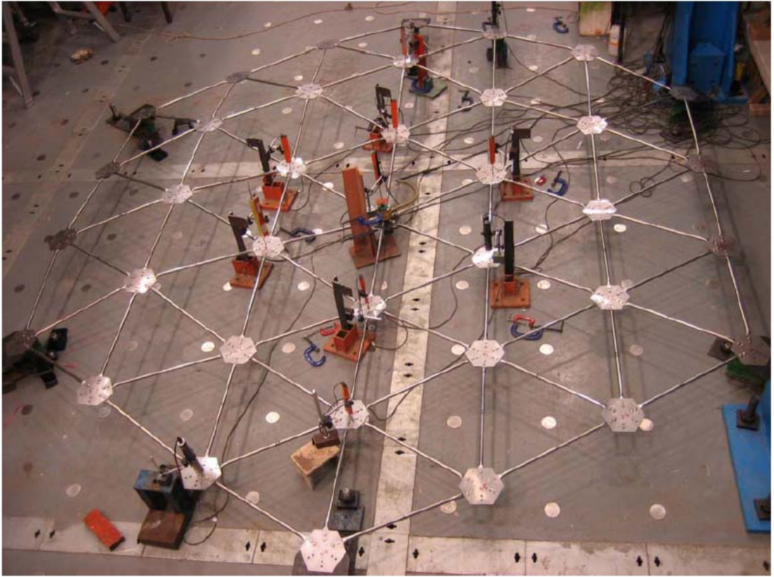
Figure 3.12 Final Deformed Shape of the Dome
