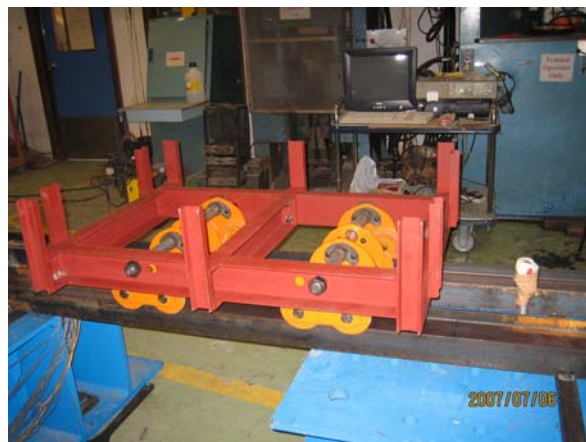
Figure 6.8 Bogie for moving vehicle simulation
