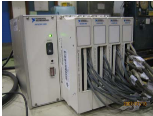
Figure 6.4 ESG data acquisition equipment
