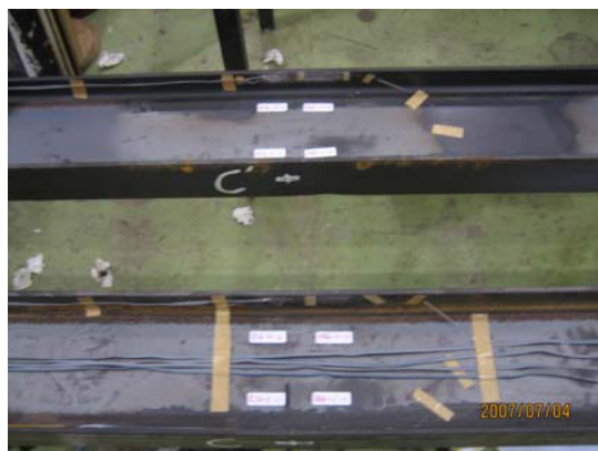
Figure 6.6 Photo of strain sensors deployed on section C
