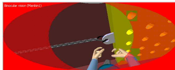
Figure 3.8: Eyesight of the worker simulated by CVP system
