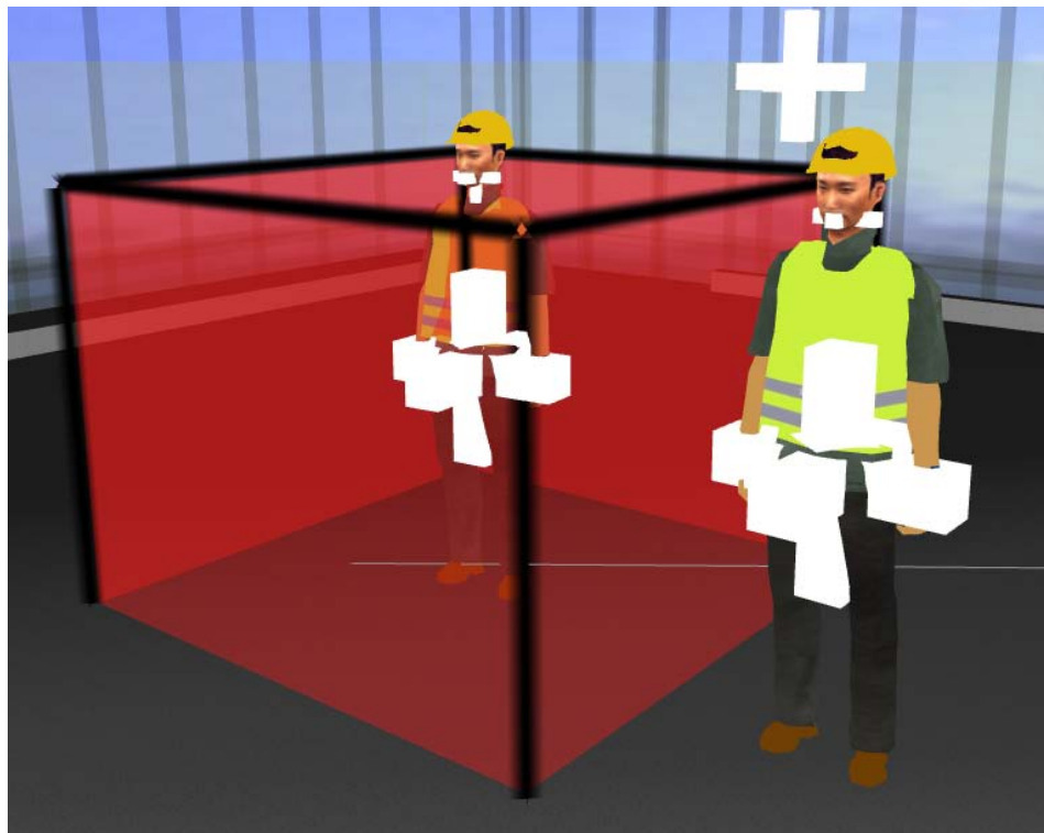
Figure 4.5. An example of a collided worker (left) and collision free worker
