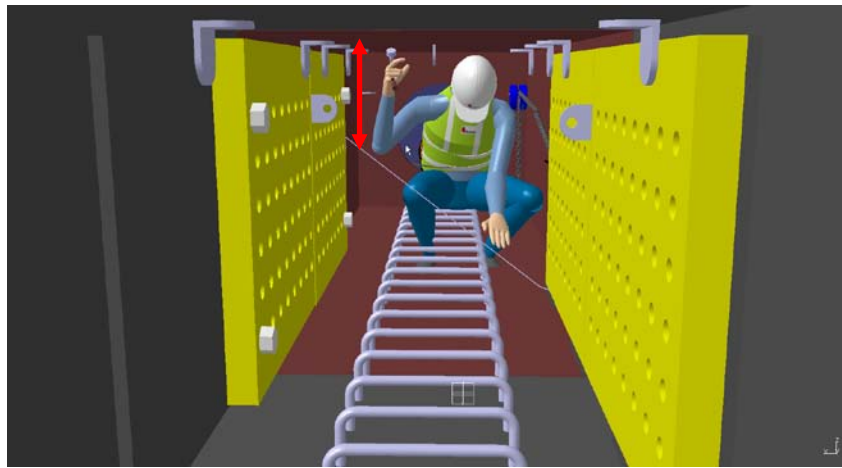
Figure 3.7: Inadequate working space within the truss
