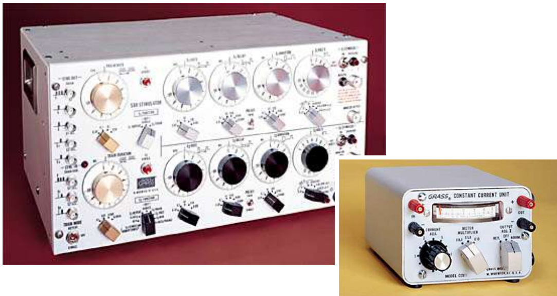
Figure 3.1 The S88K Dual Output Square Pulse Stimulator (Grass Technologies, West Warwick, RI) (left) and the Constant Current Unit (CCU) (right) (Adapted from http://www.grasstechnologies.com/products/stimulators/stimulators.html , 2010)
