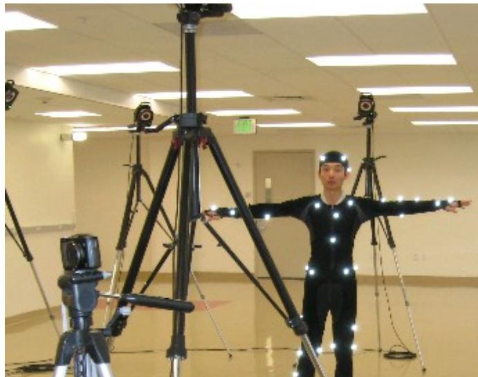
Figure 2-9. Demonstration of the Vicon Motion analysis System
