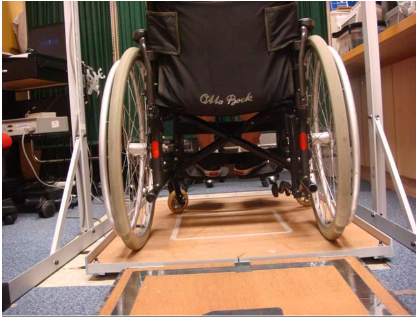
Figure 2.2 The tailor-made force platform for sitting balance control assessment
