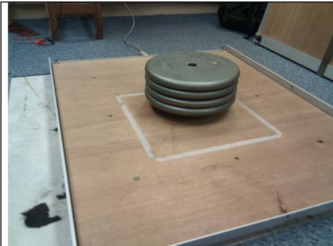
Figure H.2 Deadweight and 2 kg spacer in the center position
