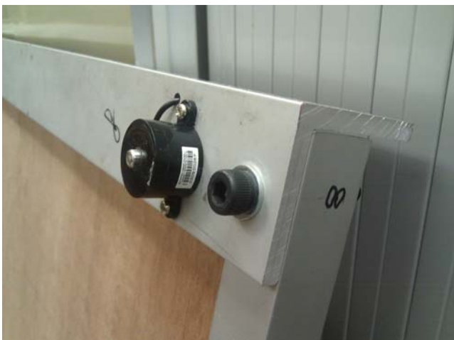
Figure H.1 The load cells are mounted on the metal frame
