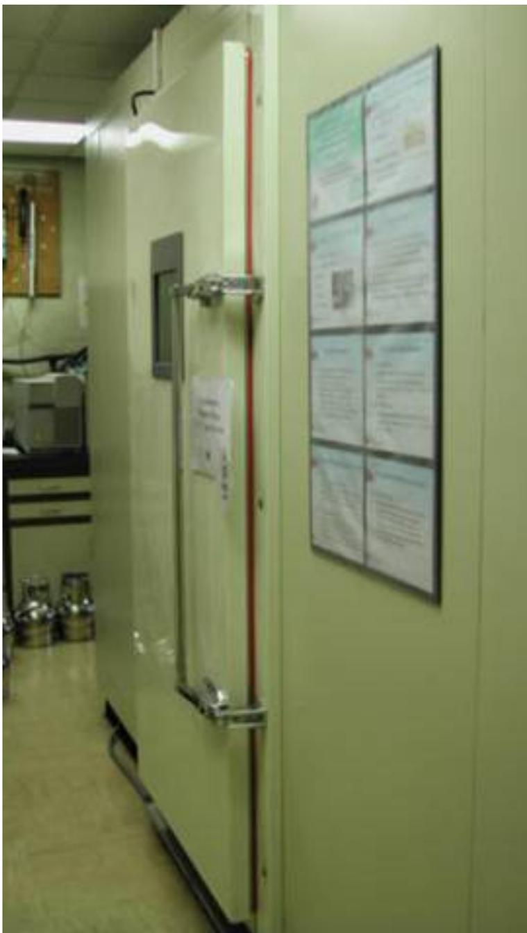
**Figure 3- 1.** A large environmental chamber
