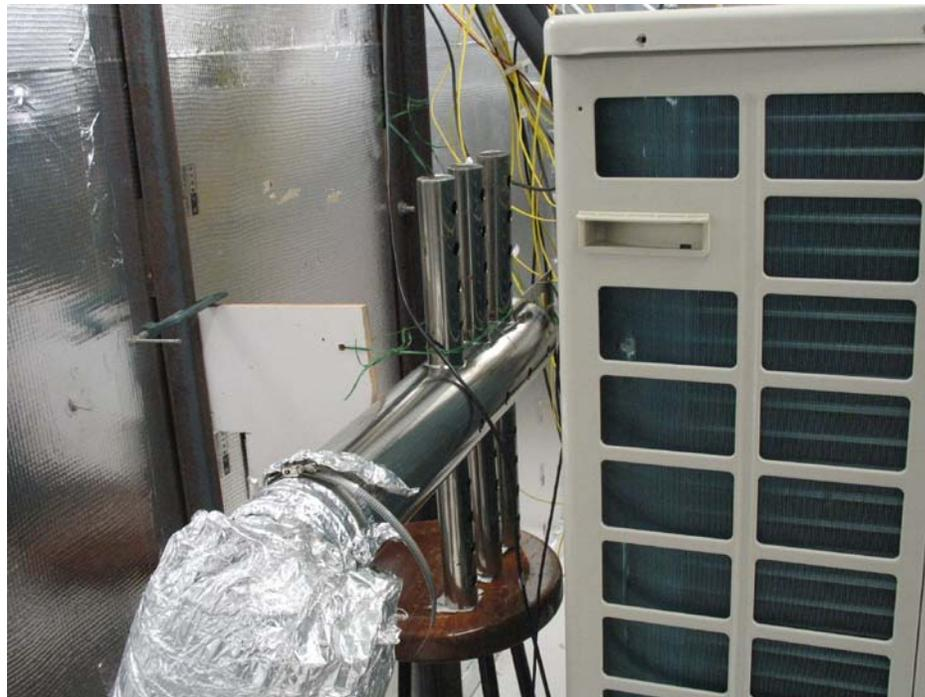
Photo 5 Air sampling device in the experimental ASPH unit (1)
