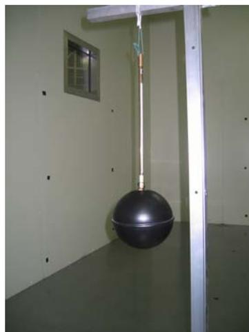
Fig. 6.5 A globe thermometer at 0.6 m height in the heated indoor space
