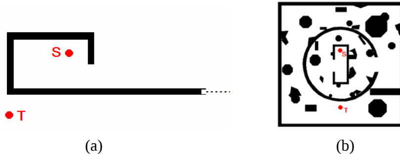
Figure 7.1: Two environment maps. S is the start of the robot, T is the goal location. (a) long-wall environment; (b) unstructured, cluttered, and maze-like environment
