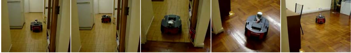
Figure 5.9: The use of linguistic commands in real world for Internet-based teleoperation. The remote operator sends a series of linguistic commands: \{GOTOEND(), TURN(180), GOTOEND(), TURN(40), MOVE(2000), TURN(90), MOVE(1000), TURN(50), MOVE(3000)\}
