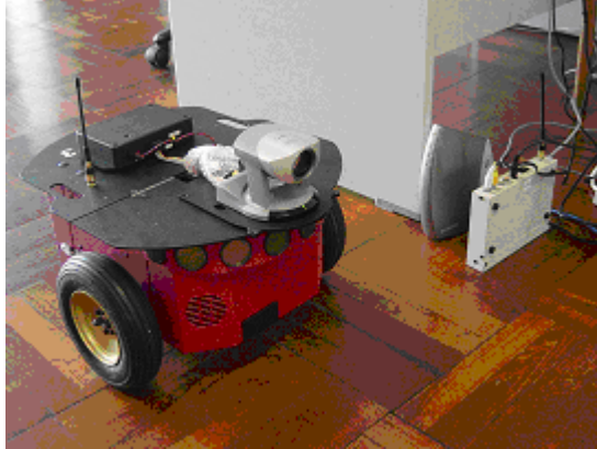
Figure 1.7: The Pioneer robot and its accessories. The robot has eight forward ultrasonic sensors and an onboard pan-tilt-zoom camera.
