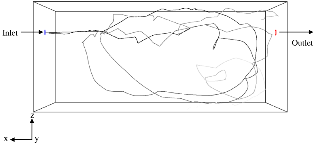
Figure 5.20: Simulated particle trajectories for inlet velocity (a) 0.17 \text{ ms}^{-1} and (b) 1.8 \text{ ms}^{-1}
