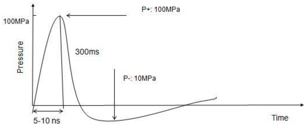
Figure 1.1 Graphic representation of a shock wave. There is a very rapid pressure rise ( $<10\text{ns}$ ) to a high peak pressure ( $>10\text{MPa}$ ), followed by a variable negative pressure, which may cause cavitation.
