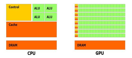
Figure 2.3 - The GPU Devotes More Transistors to Data Processing [12]
