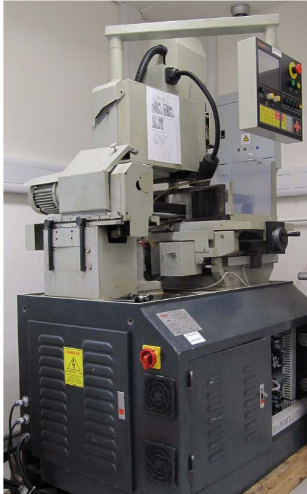
Fig. 2.3 Photograph of WEDM equipment used to prepare our [112]-oriented Terfenol-D short bars in Fig. 2.2.
