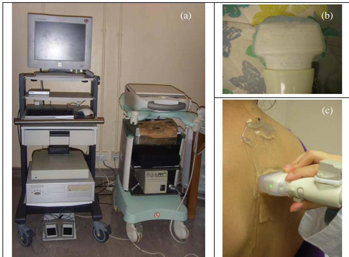
Figure 3. 4. 3-D Ultrasound System (a) Ultrasound Unit and 3-D Add-on System (b) Probe of Ultrasound Unit with a Silicone Sleeve (c) The Probe in Ultrasound Scanning Procedure
