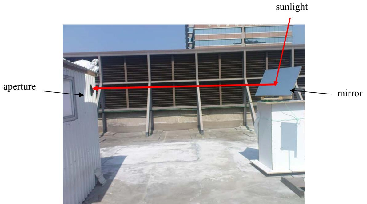
Fig. 6.6 Mirror reflected sunlight into the RSSL
