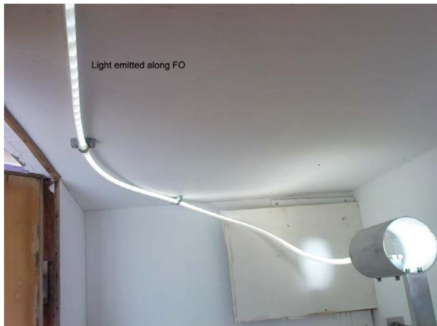
Fig. 6.7 Light emitted along notched fiber optic
