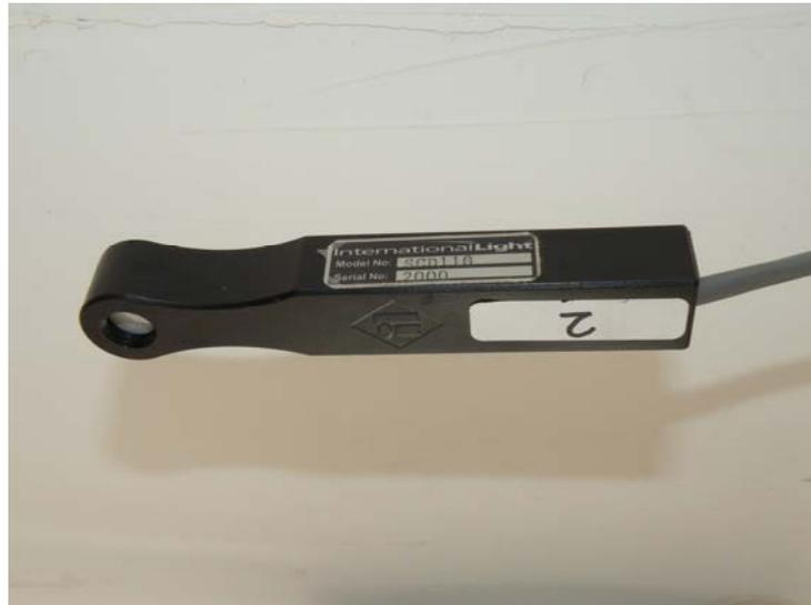
Fig. 6.9 The indoor light sensor
