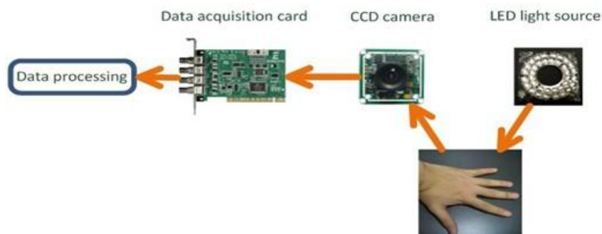
Figure 5.1: The schematic diagram of the developed hand back skin texture imaging system.
