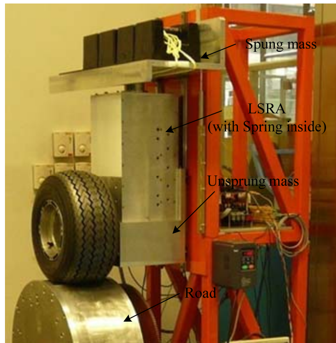
Fig. 6-2 Experimental setup of quarter-vehicle model
