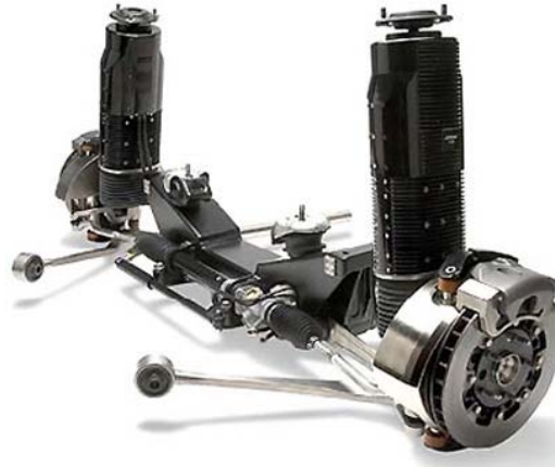
Fig. 1-3 The Bose® electromagnetic active suspension
