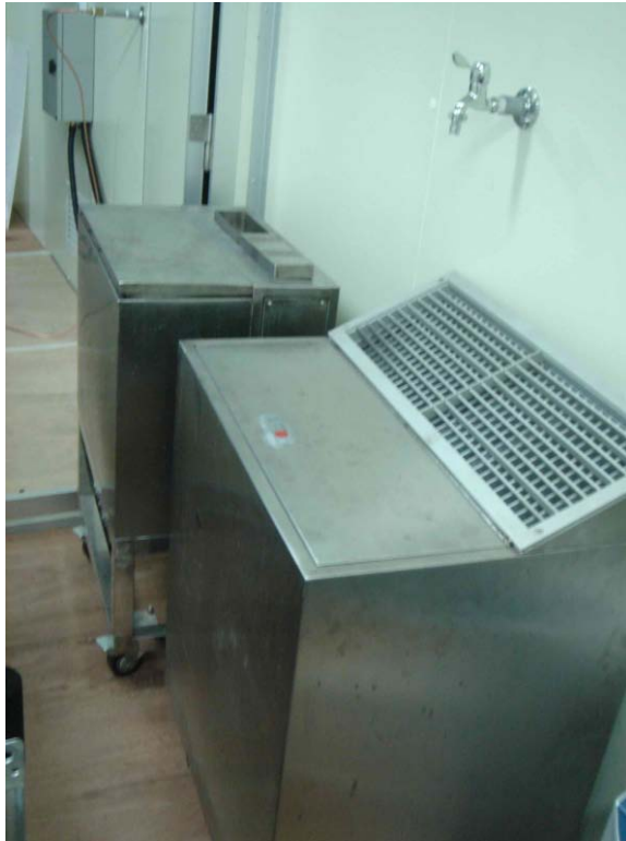
Photo 5 Load generation units inside conditioned space
