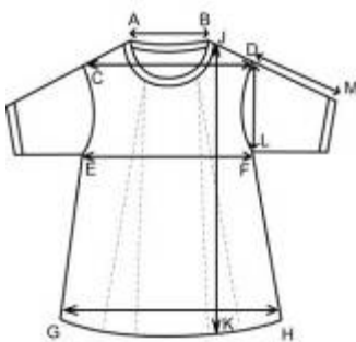
Figure 6.4 – Shape and measurements of T-shirts (F-1 and F-2)
