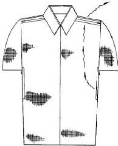
Figure 3.4 - Convectively ventilated garments having protective shield layers.
