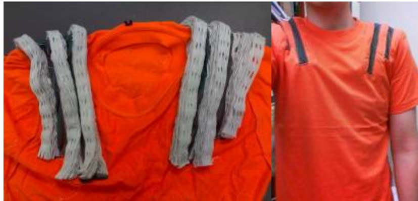
Figure 8.2 – Spacer shoulder pad. (Left: inner construction; right: the T-shirt)
