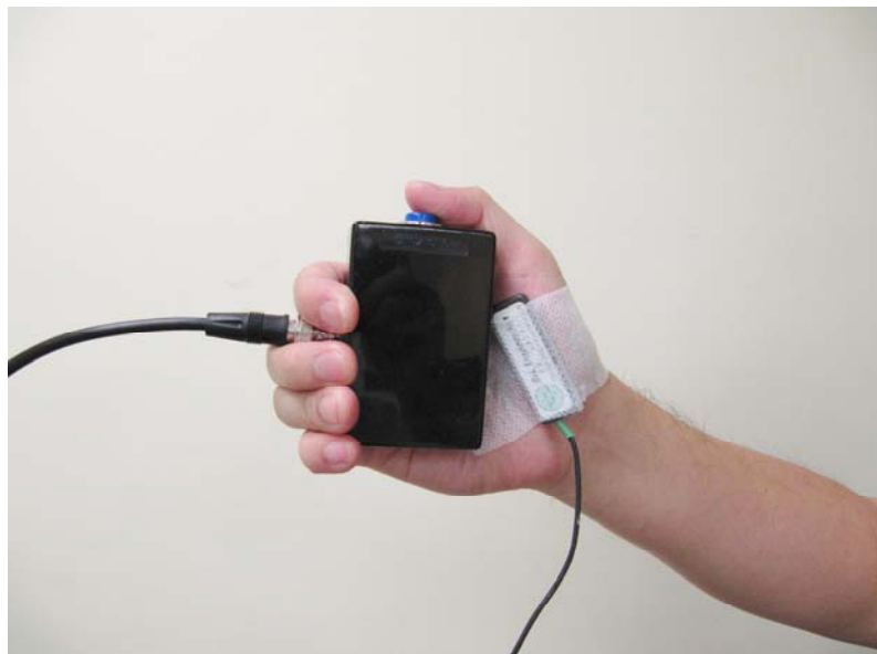
Figure 6. Electrode placement on the flexor pollicis brevis
