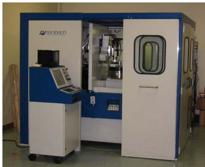
Figure 2.8 Freeform 705G ultra-precision five axis raster milling machine
