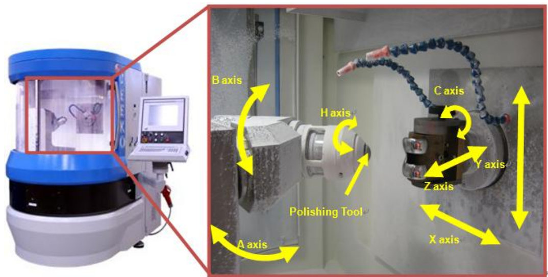
Figure 2.10 IRP200 Ultra-precision multi-axis freeform polishing machine
