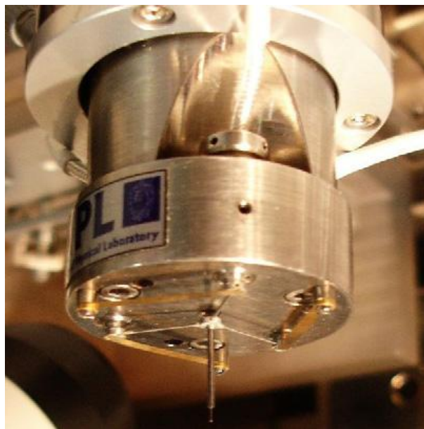
Figure 2.15 Micro probing system developed by NPL (Adapted from Peggs et al, 1999)
