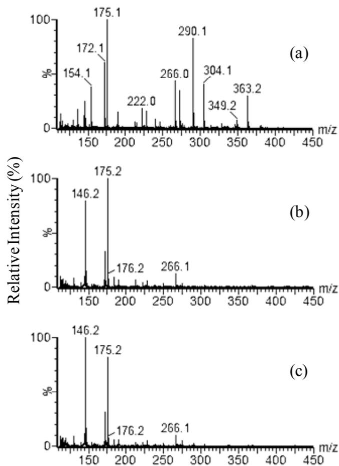
**Figure 2.15.** MALDI-MS spectra for *Panax ginseng* obtained by: (a) analysis of the extract of sample powder with matrix solution (10 mg/mL CHCA in 50/50 ACN/H<sub>2</sub>O with 0.1% TFA) as the extraction solvent, (b) direct analysis of sample powder with CHCA (10 mg/mL in 100% acetone) as the matrix solution, and (c) analysis of the extract of sample powder with matrix solution (10 mg/mL CHCA in 100% acetone with 0.1% TFA) as the extraction solvent.
