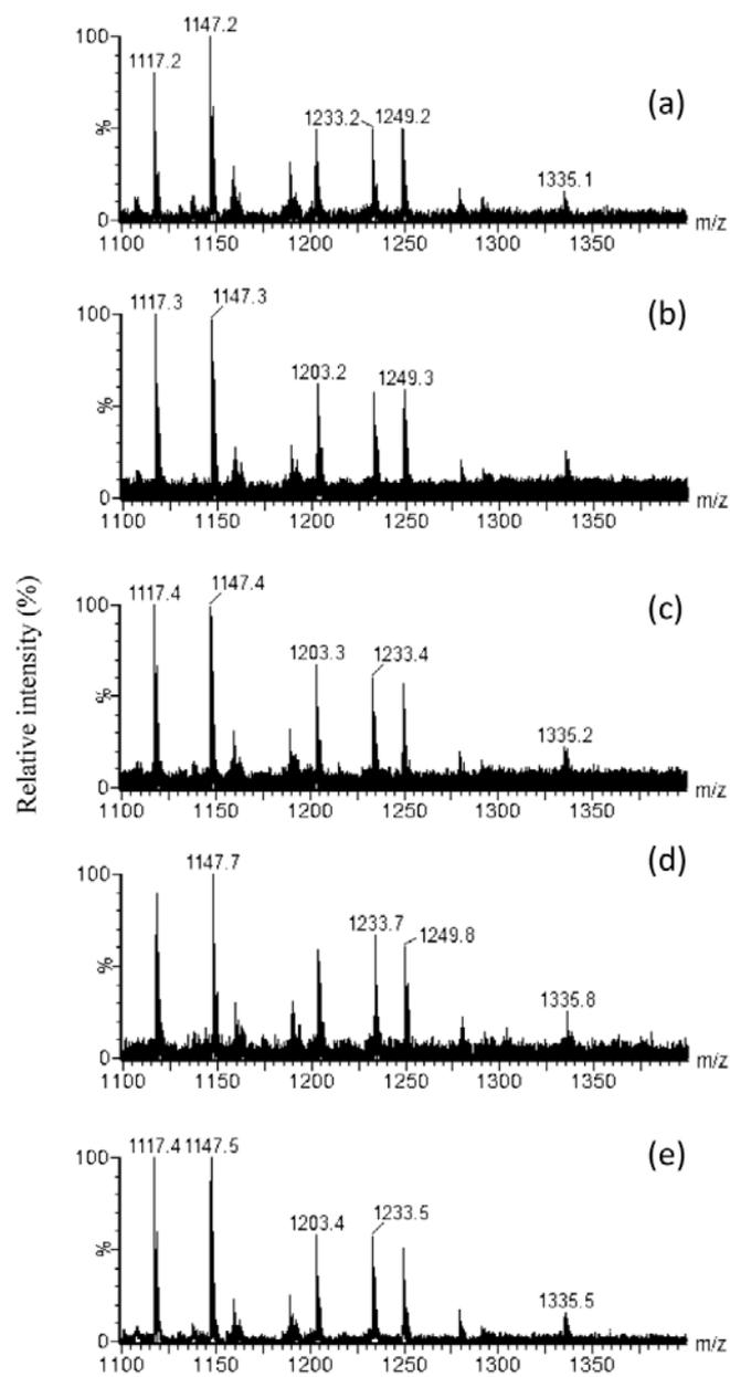
**Figure 2.1.** MALDI-MS spectra obtained for *Panax ginseng* in high mass region with different solvent extractions (a) 50% ACN, (b) 50% MeOH, (c) 100% H<sub>2</sub>O, (d) 100% ACN, (e) 100% MeOH. All the solvents contained 0.1% TFA. Mass peaks from CHCA matrix are labeled with "\*".
