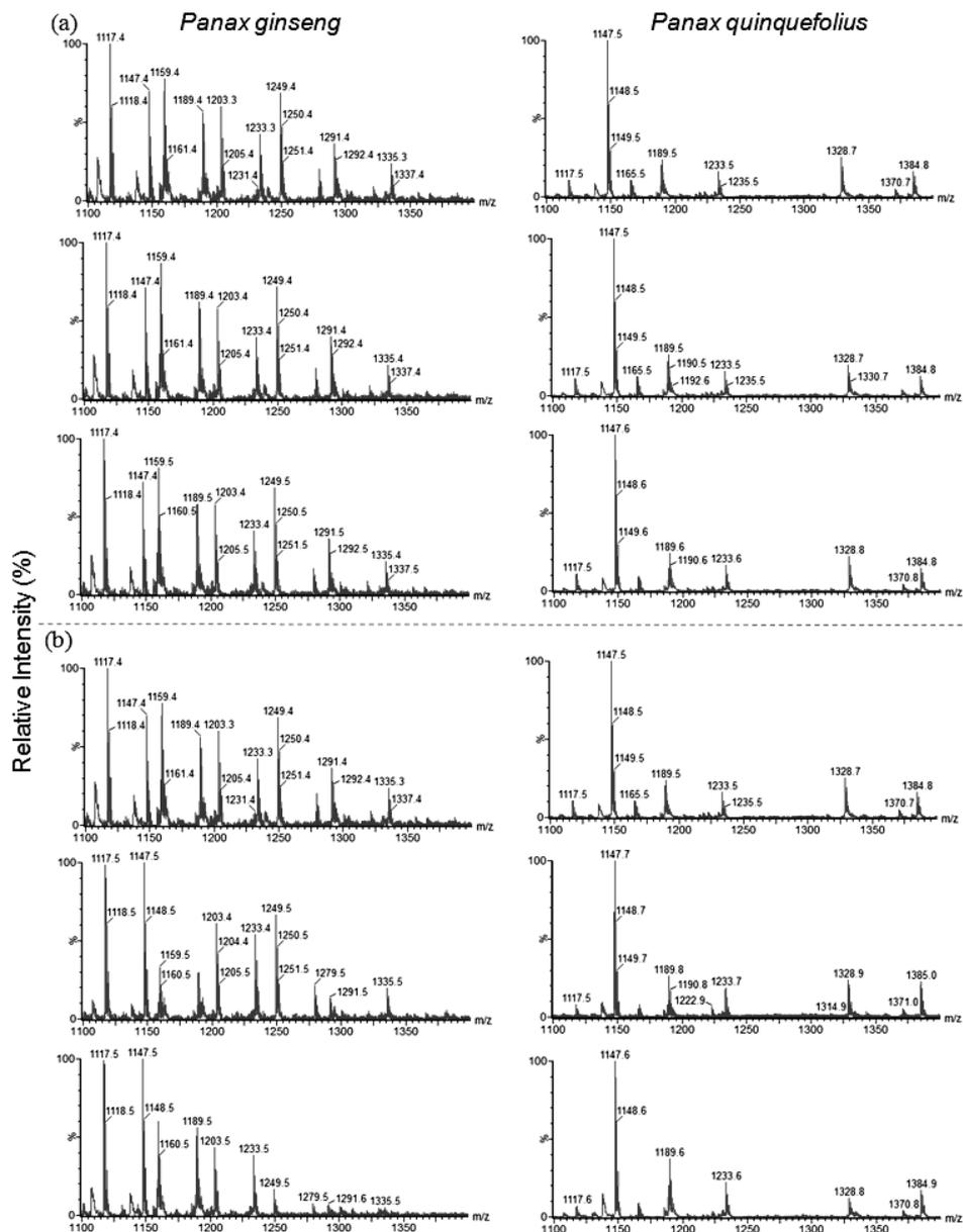
**Figure 2.6.** Test for reproducibility of the mass spectra obtained for *Panax ginseng* (left column) and *Panax quinquefolius* (Canada) (right column) acquired in the high mass region. (a) MALDI-MS spectra of the same herb samples obtained in three independent experiments. (b) MALDI-MS spectra obtained for the same species of herb samples purchased from three different pharmacies.
