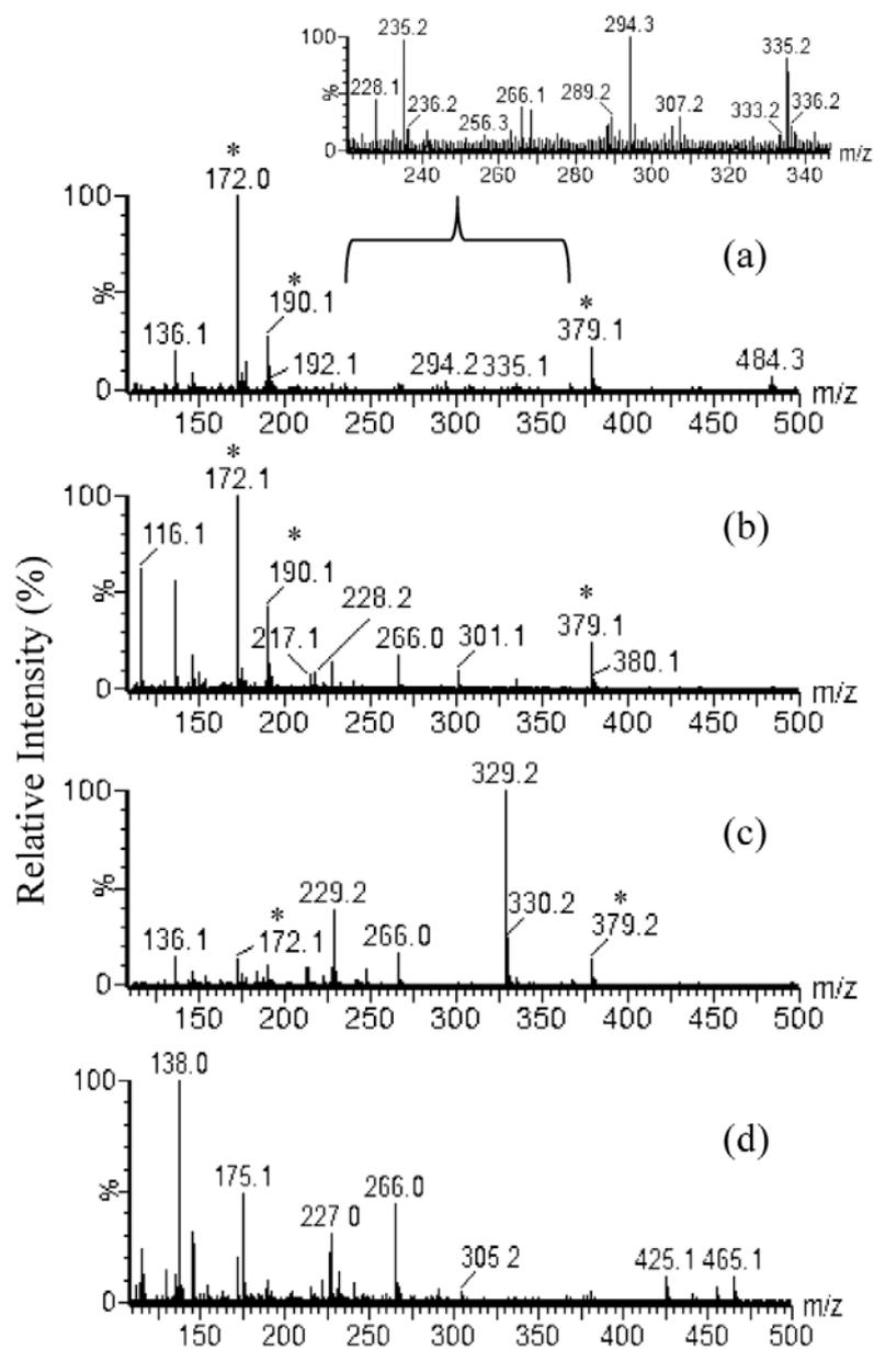
**Figure 4.3.** MALDI-MS spectra of *Angelica* roots from different harvesting locations: (a) *A. sinensis*, (b) *A. acutiloba*, (c) *A. archangelica* L. and (d) *A. gigas*. Mass peaks from the CHCA matrix are labeled with “\*”.
