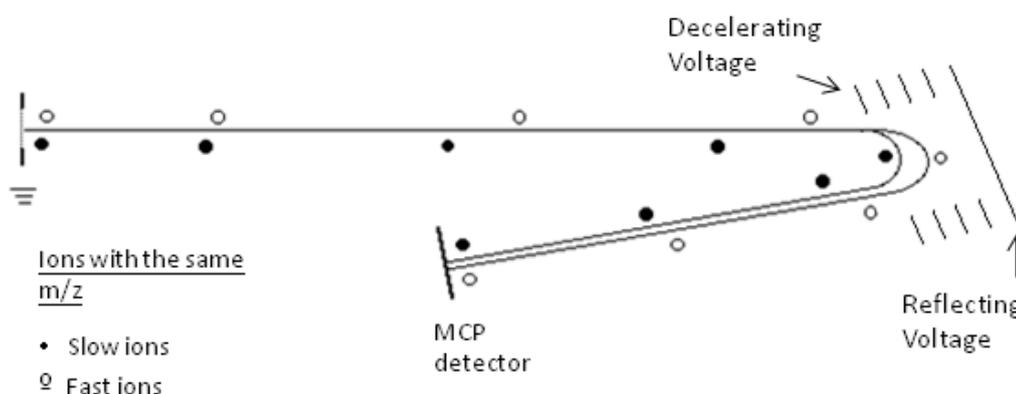
**Scheme 1.2** Schematic diagram showing the ion pathways in the reflectron-TOF analyzer.
