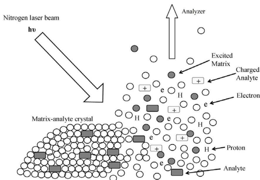
**Scheme 1.1** Schematic diagram of the MALDI ionization process.<sup>46</sup>
