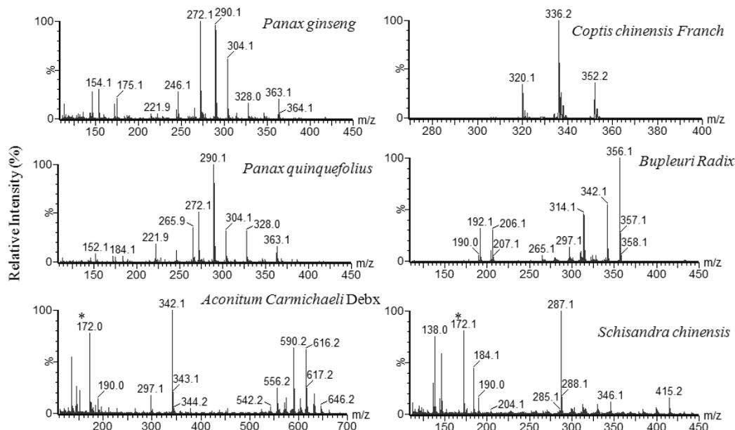
**Figure 2.10.** MALDI-MS spectra of different TCM herbs acquired in the low mass region. Mass peaks from CHCA matrix are labeled with "\*".
