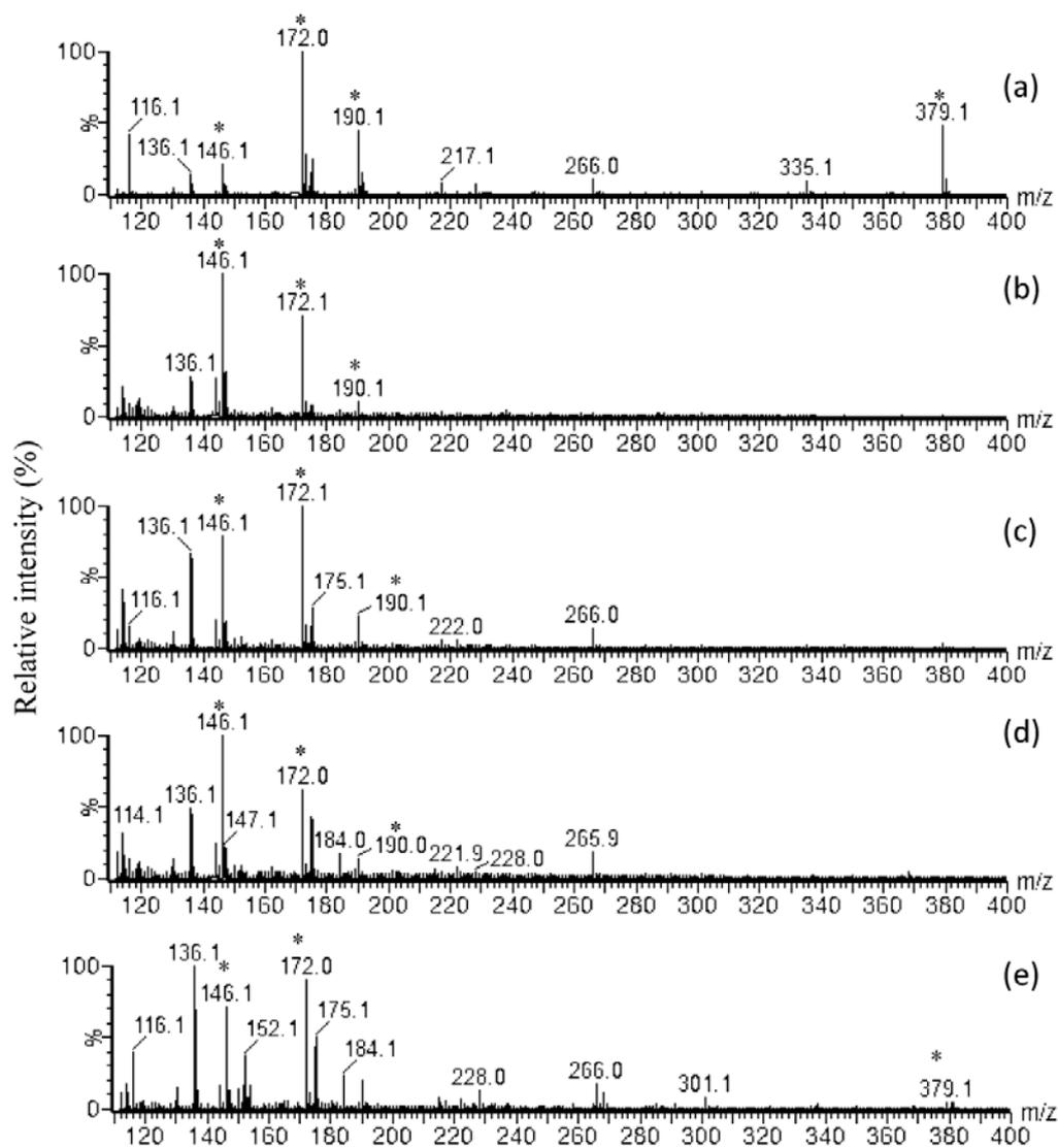
**Figure 4.1.** MALDI-MS spectra obtained for *A. acutiloba* with different extraction solvents: (a) 50% ACN, (b) 50% MeOH, (c) 100% H<sub>2</sub>O, (d) 100% ACN and (e) 100% MeOH. All solvents contained 0.1% TFA. Mass peaks from the CHCA matrix are labeled with "\*".
