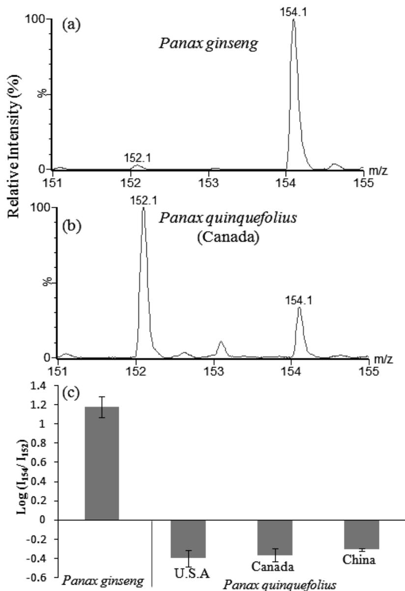
**Figure 2.11.** MALDI-MS spectra showing the relative abundance of the m/z 154 and m/z 152 components detected for *Panax ginseng* (a) and *Panax quinquefolius* (b) respectively. (c) A chart showing the logarithm of the intensity ratio of m/z 154 to m/z 152 ( $I_{154}/I_{152}$ ).
