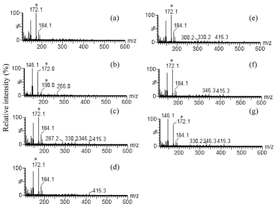
**Figure 3.2.** MALDI-MS spectra obtained for *S. sphenanthera* with different extraction time: (a) 0 min; (b) 1 min; (c) 3 min; (d) 10 min; (e) 20 min; (f) 40 min and (g) 60 min. Mass peaks from the CHCA matrix are labeled with "\*".
