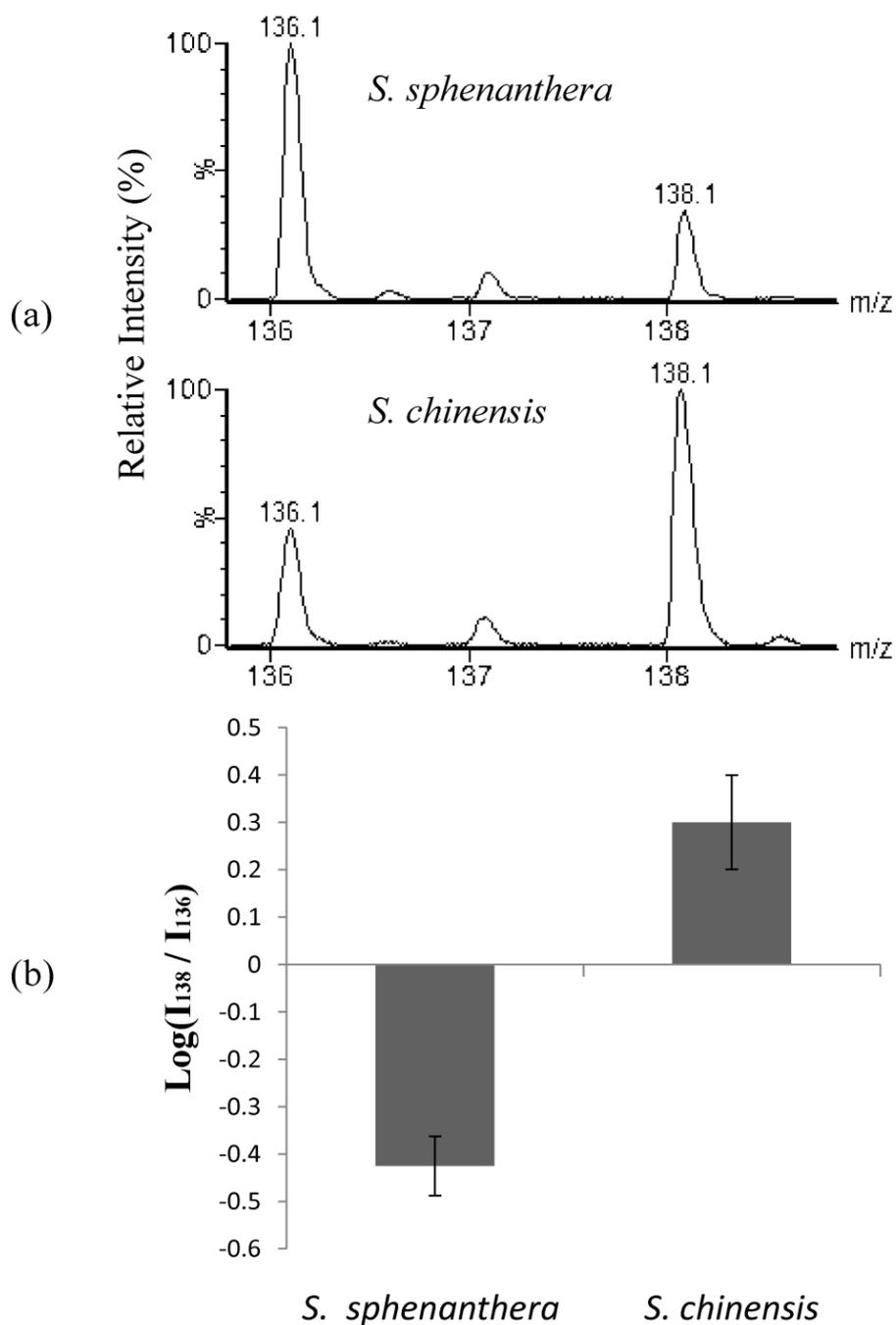
**Figure 3.9.** (a) MALDI-MS spectra at mass range of 136 -138 Da for *S. sphenanthera* and *S. chinensis*. (b) Plot for logarithm of  $I_{138}/I_{136}$  against the *Fructus Schisandrae* sample.
