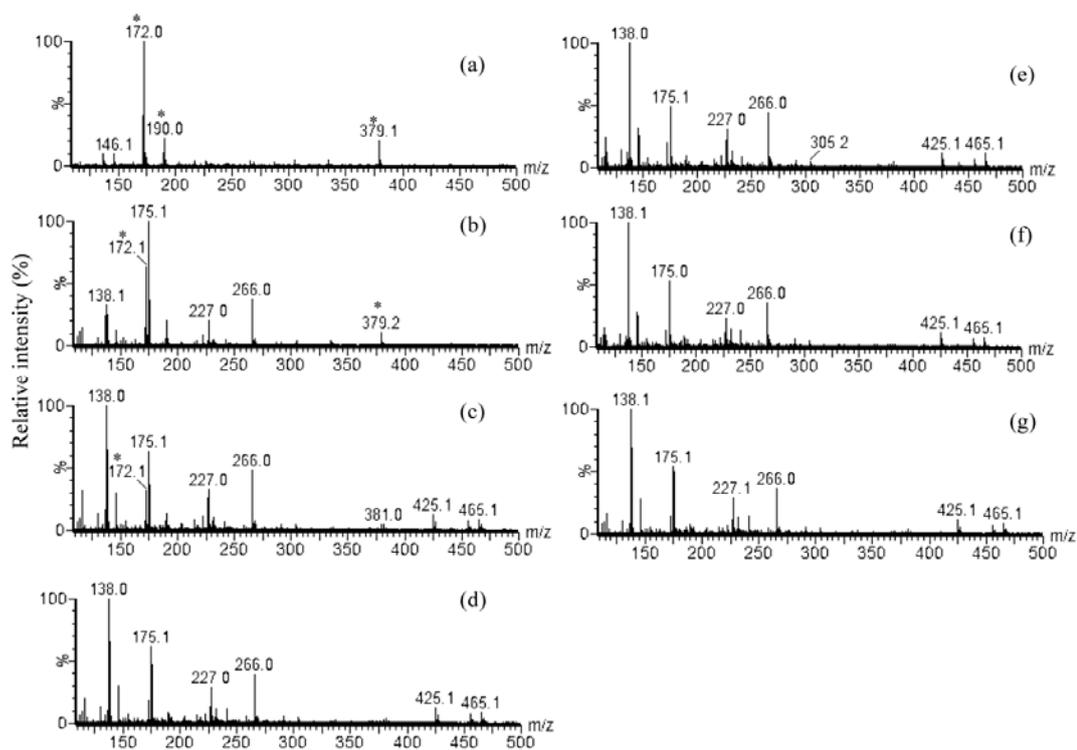
**Figure 4.2.** MALDI-MS spectra obtained for *A. archangelica L.* with different sonication time: (a) 0 min, (b) 1 min, (c) 3 min, (d) 10 min, (e) 20 min, (f) 40 min and (g) 60 min. Mass peaks from the CHCA matrix are labeled with "\*".
