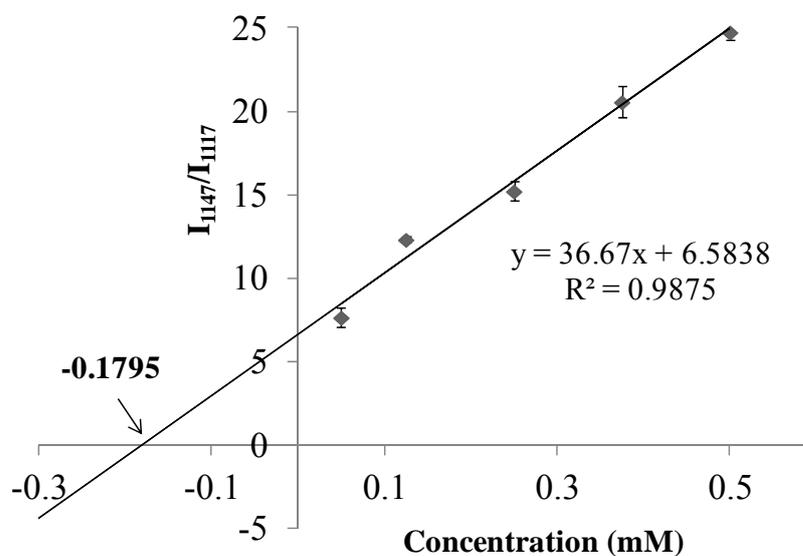
**Figure 2.13.** Plot of  $I_{1147}/I_{1117}$  against the added ginsenoside Rb1 standard concentration in the ginseng extract.
