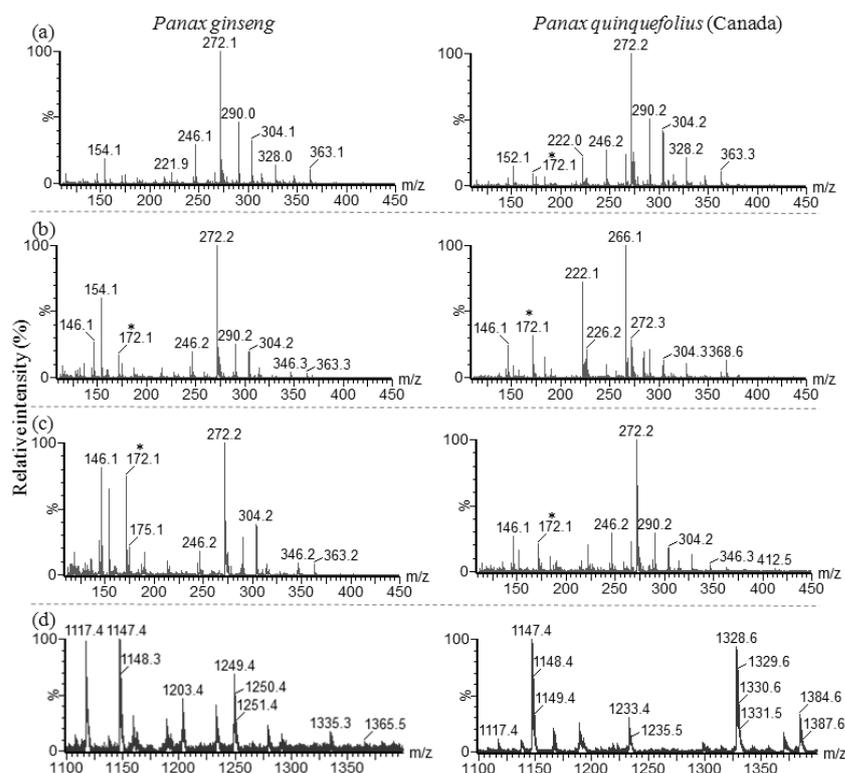
**Figure 2.14.** MALDI-MS spectra obtained for *Panax ginseng* (left column) and *Panax quinquefolium* (right column) using different solid sample preparation methods. (a) – (c): Mass spectra acquired in low mass region using the powder, slice, and sandpaper method, respectively. Mass peaks from CHCA matrix are labeled with "\*". (d): Mass spectra acquired in high mass region using the powder method.
