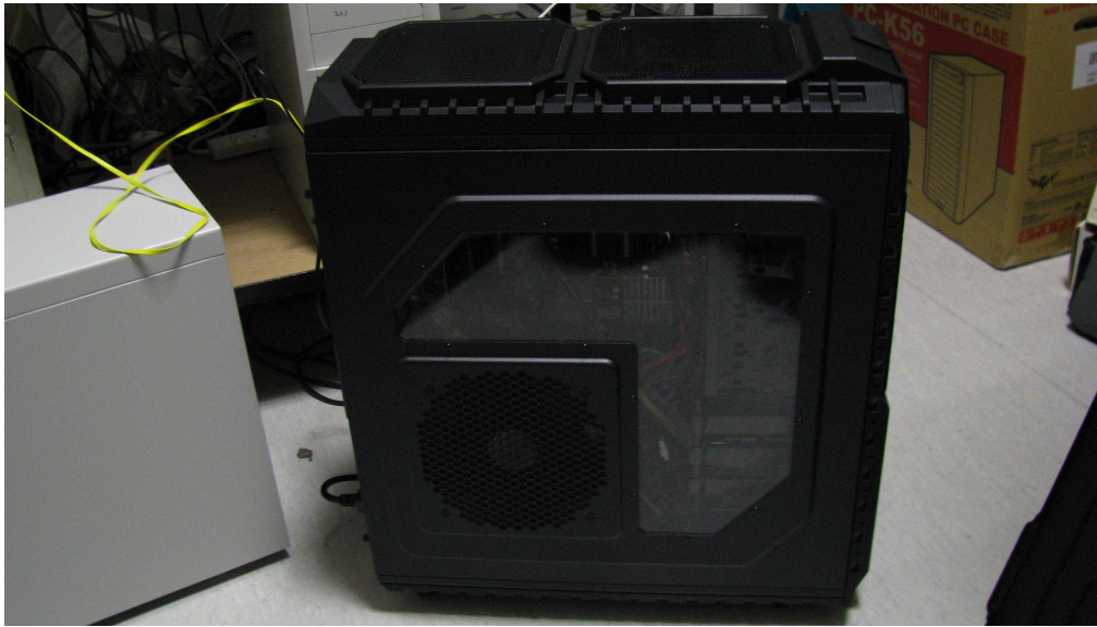
Fig. 2.5 – Two additional fans on the top and 1 additional fan on the side cover to ensure satisfactory cooling.
