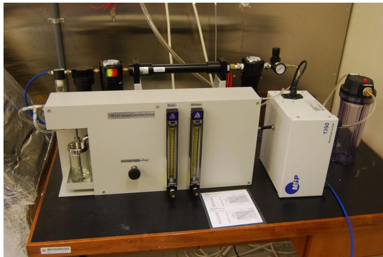
Figure 3.3 Particle generation system
